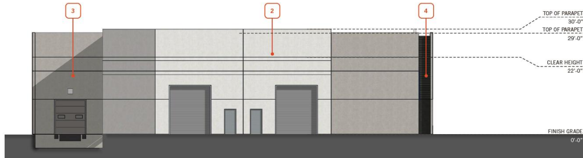
BUILDING 5 EAST ELEVATION - SCALE: 1/8" = 1'-0"
