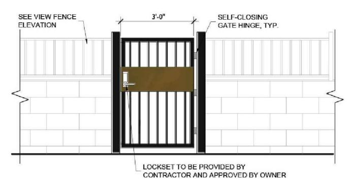
EXTERIOR PEDESTRIAN GATE - ELEVATION
