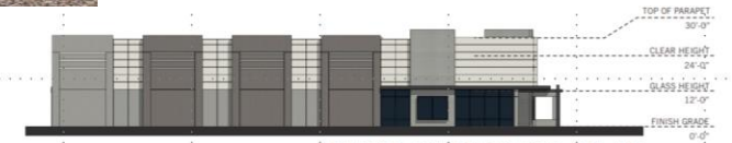
BUILDING 3 - NORTH ELEVATION - SCALE: 1/16" = 1'-0"
