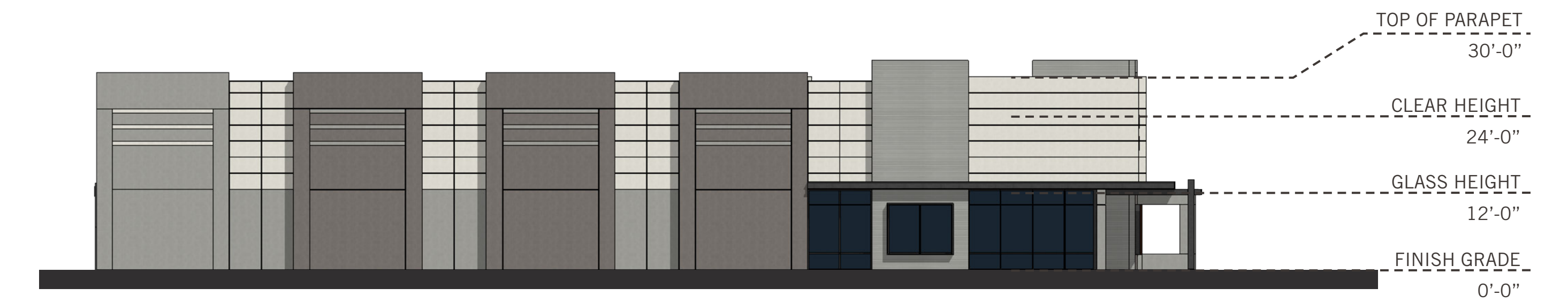
BUILDING 3 - NORTH ELEVATION - SCALE : 1/16" = 1'-0"
