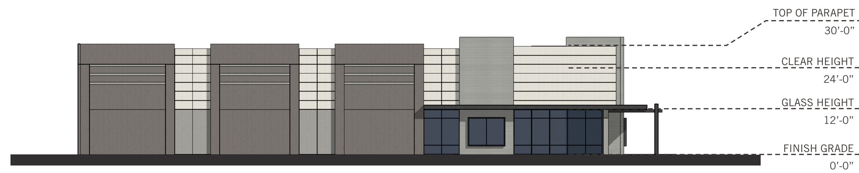
BUILDING 1 - NORTH ELEVATION - SCALE : 1/16" = 1'-0"
