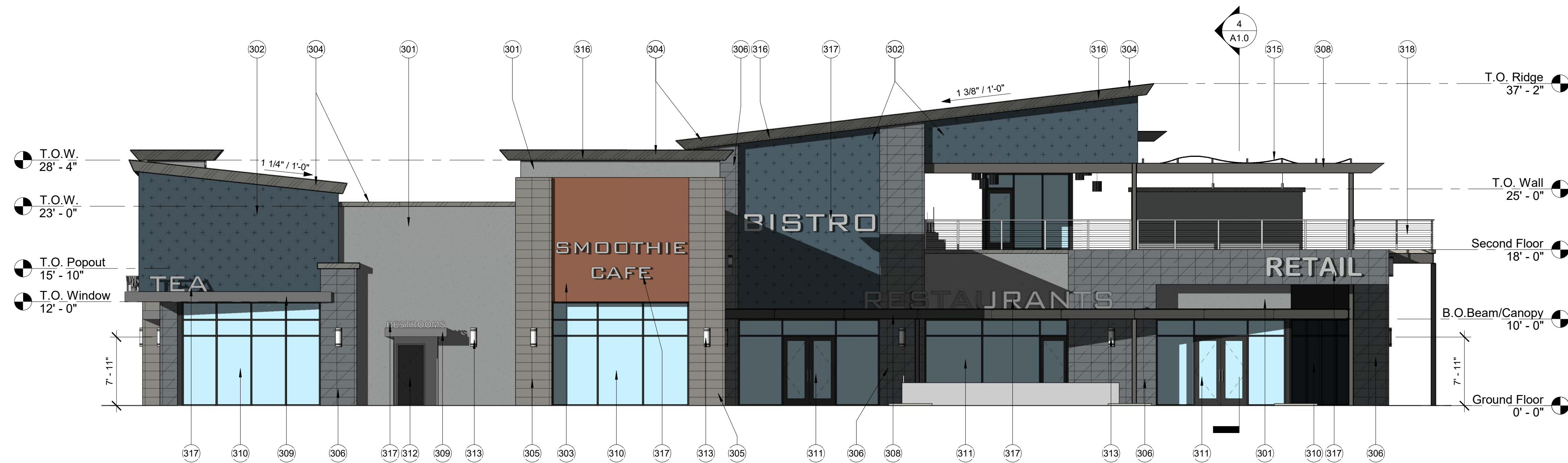
1 East Elevation - Building A 1/8" = 1'-0"
