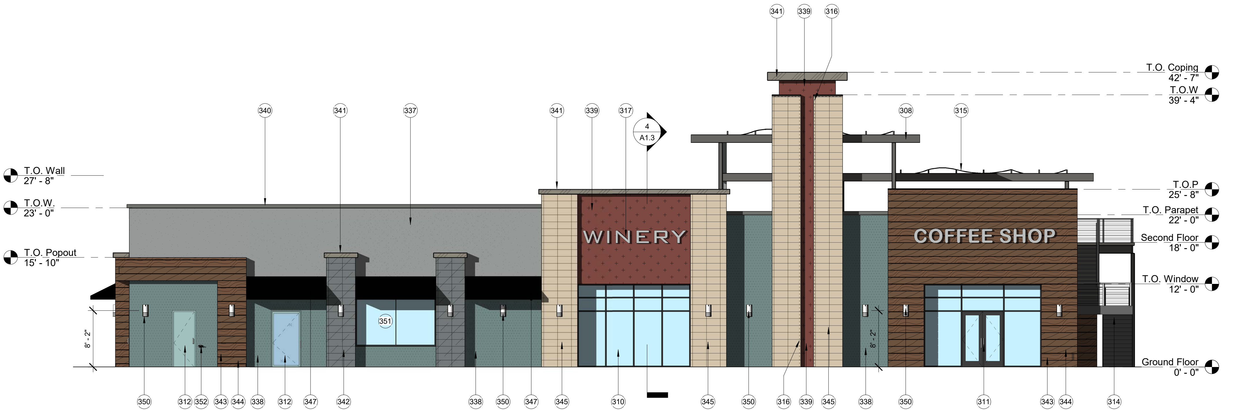
1 East Elevation - Building D 1/8" = 1'-0"
