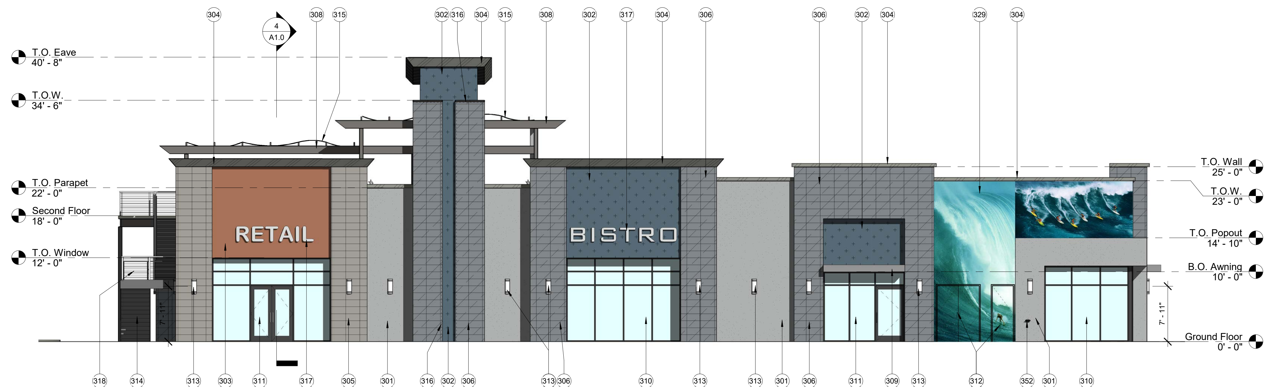
2 West Elevation - Building A 1/8" = 1'-0"
