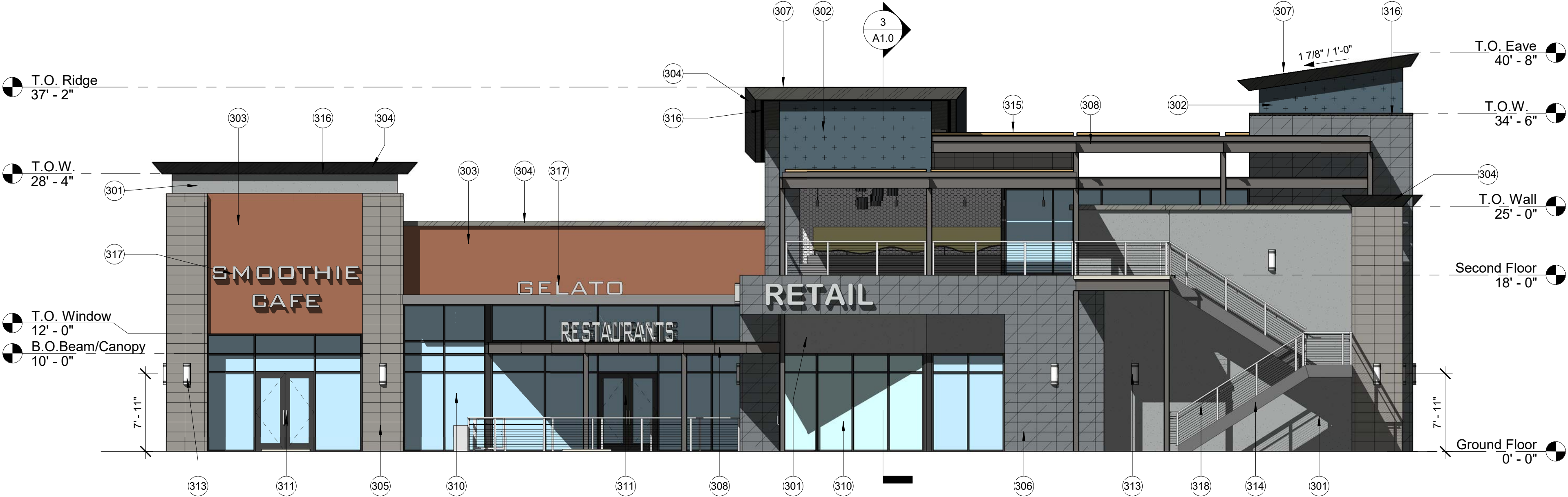
1 North Elevation - Building A 1/8" = 1'-0"
