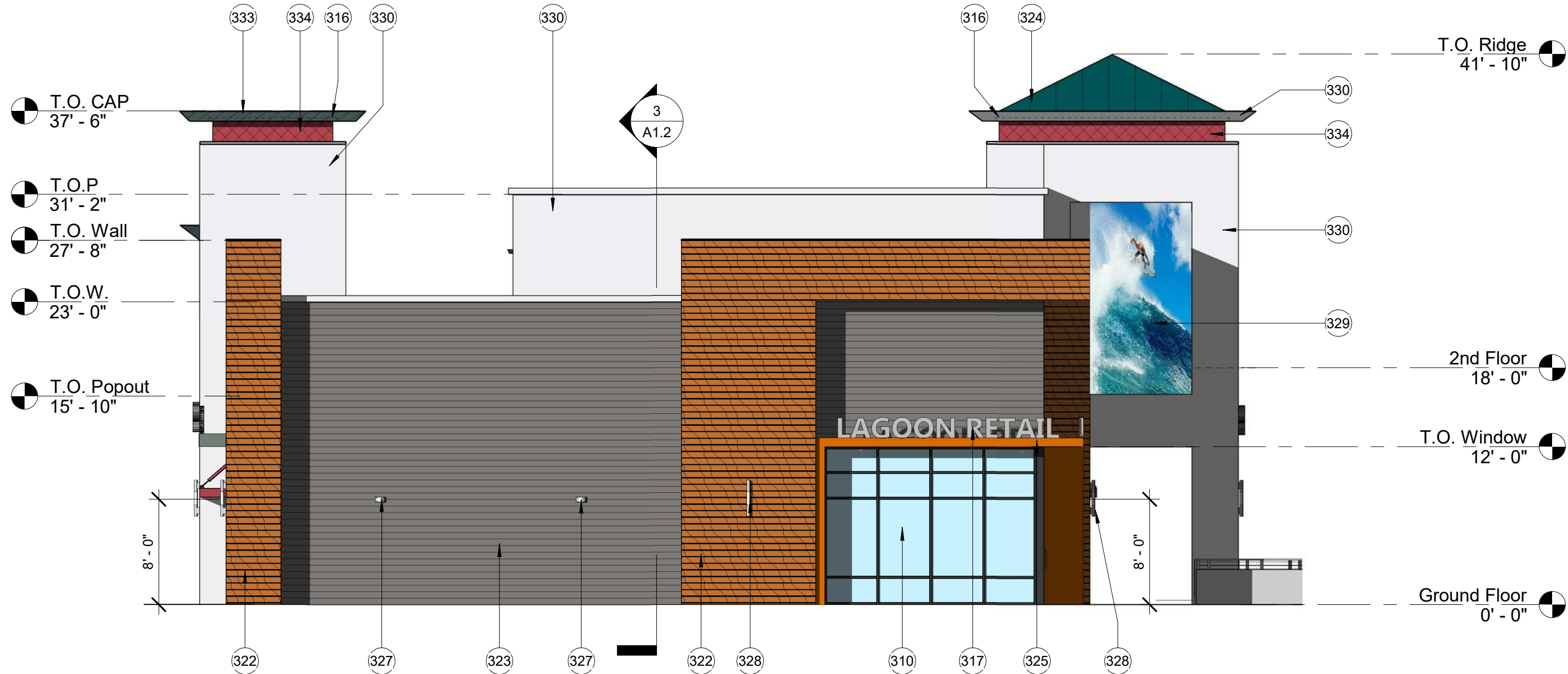
1 East Elevation - Building C 1/8" = 1'-0"
