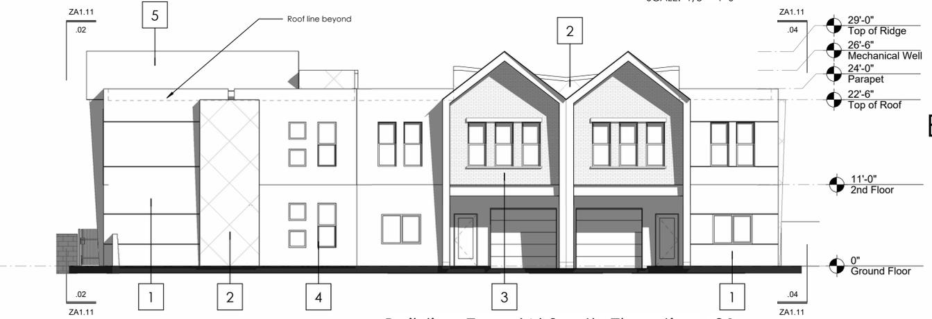
Building Type 'A' South Elevation .01
