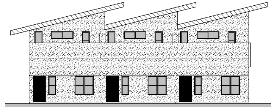
EAST ELEVATION 1391sf STUCCO 1046sf / 1391sf = 75% METAL 98sf / 1391sf = 7% GLAZING 177sf / 1391sf = 13% DOORS 70sf / 1391sf = 5%
