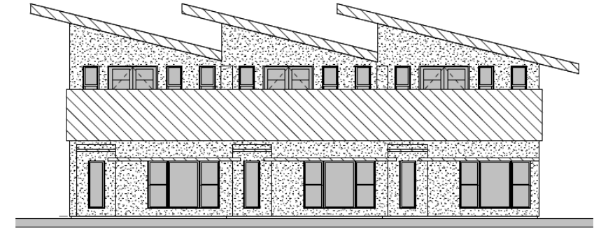
WEST ELEVATION 1397sf STUCCO 580sf / 1397sf = 42% METAL 509sf / 1397sf = 36% GLAZING 308sf / 1397sf = 22%
