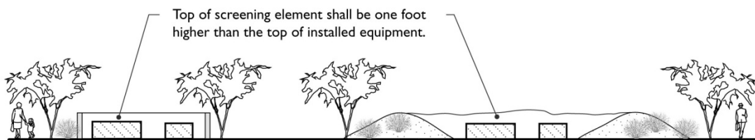
Figure 8.8.(h)(i) : Screening of Ground-Mounted Equipment
