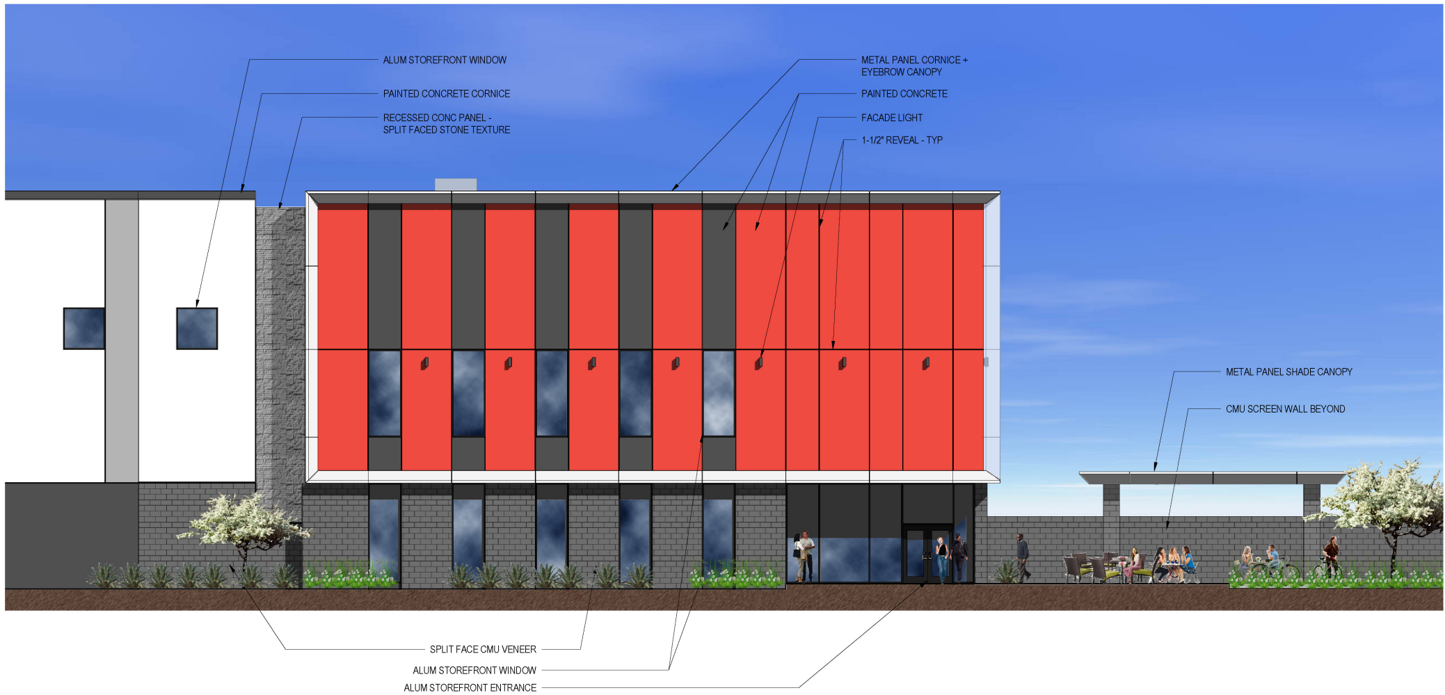
ELEVATION DETAIL - WEST 1/8" = 1'-0"
