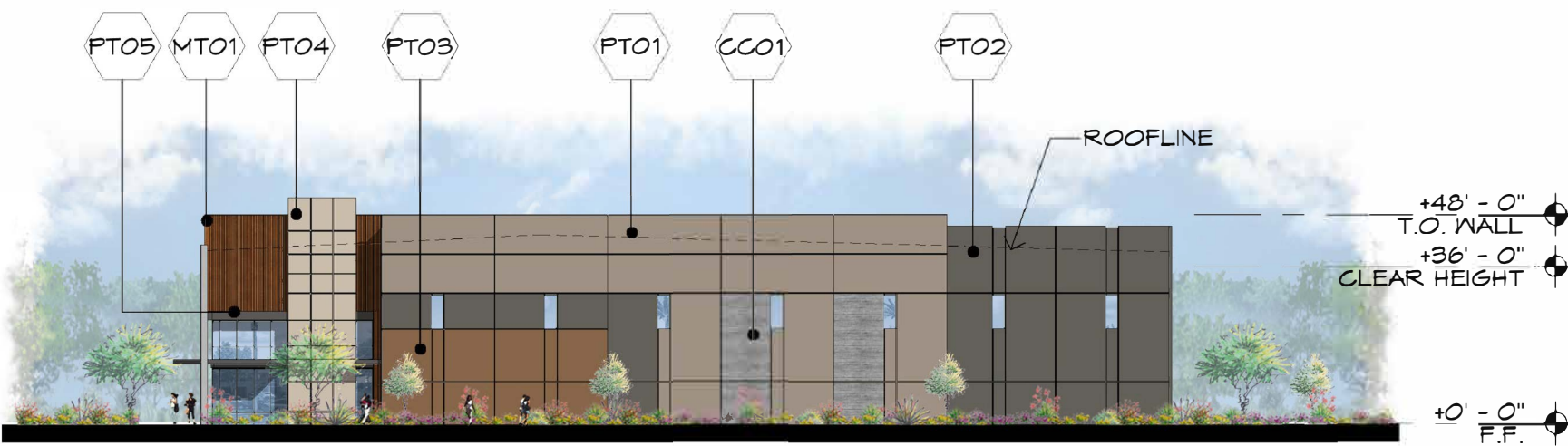
2 BUILDING A WEST ELEVATION SCALE: 1" = 40'-0"
