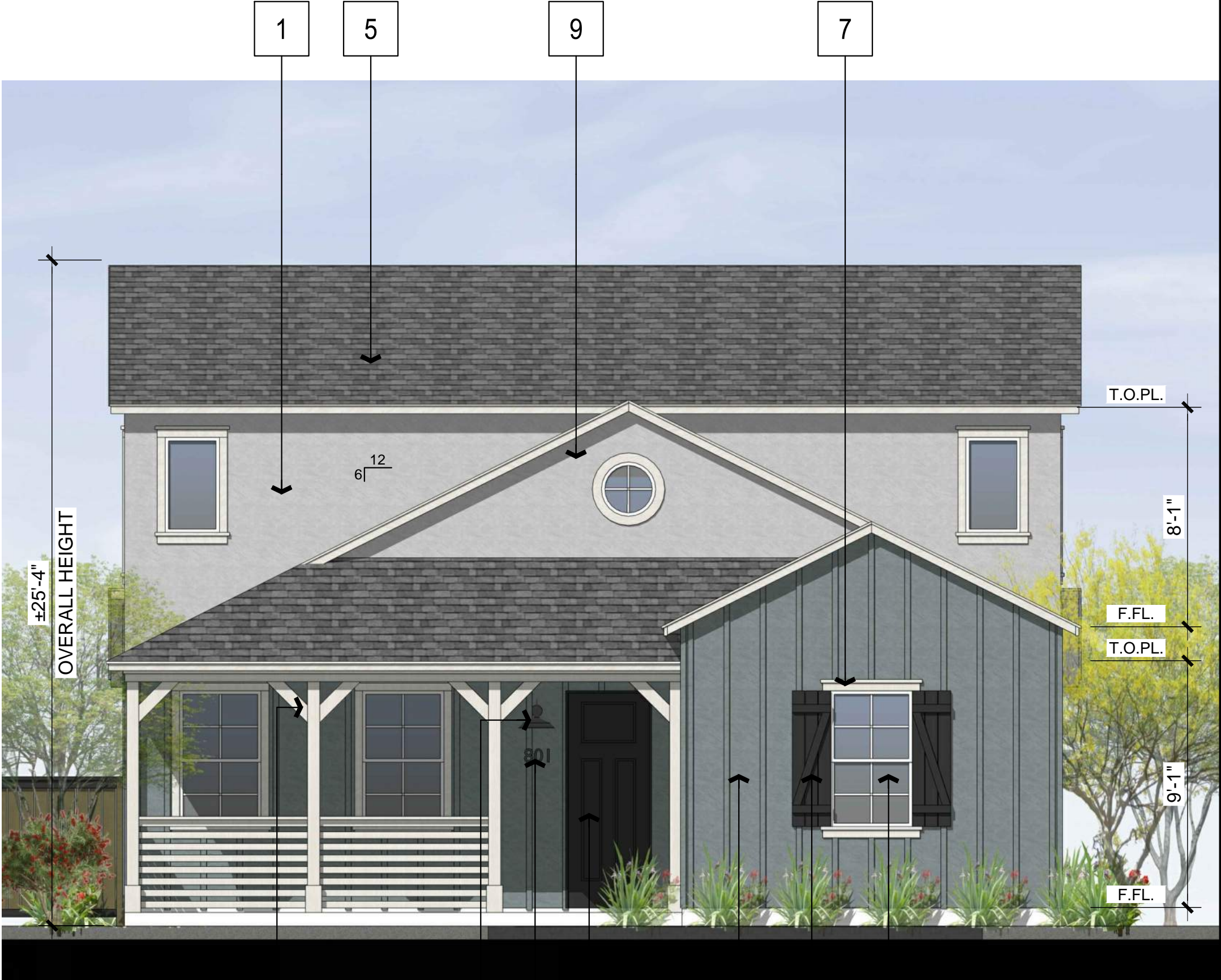
8 10 11 2 3 6 4 FRONT MATERIAL PERCENTAGE SIDING:269 SQ. FT. = 62% STUCCO:168 SQ. FT. = 38% TOTAL:437 SQ. FT.
