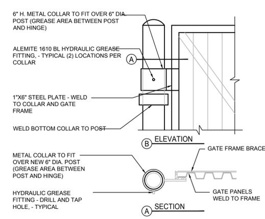
1 GATE HINGE @ TRASH SCALE: 1" = 1'-0"
