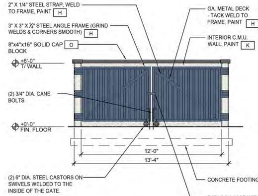
5 TRASH GATE ELEVATION SCALE: 1/4" = 1'-0"
