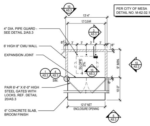
6 TRASH ENCLOSURE PLAN SCALE: 1/8" = 1'-0"
