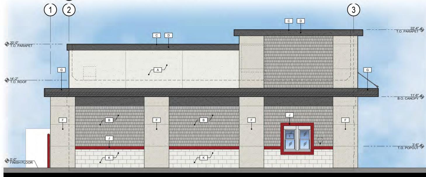
2 SOUTH ELEVATION (DRIVE-THRU WALL)
