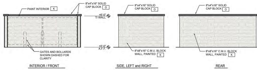
10 TRASH ENCLOSURE ELEVATIONS SCALE: 1/4" = 1'-0"
