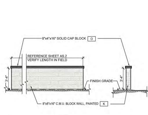
9 CONCRETE SCREEN WALL ELEVATION SCALE: 1/4" = 1'-0"
