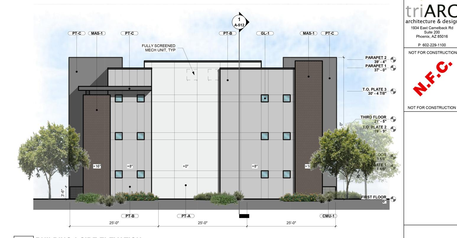
**BUILDING 2 SIDE ELEVATION** 2 BUILD **BUILDING 2 SIDE ELEVATION MATERIALS** STUCCO = 1965 SF (77%) GLAZING EXPOSED CMU = 48 SF (2%) = 26 SF (1%) BRICK VENEER = 525 SF (20%)
