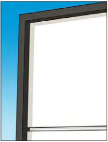
PANEL DETAIL Panel Faces Inset 2" From Accent Frame Face
