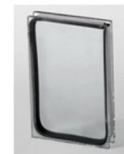
GL - GLAZING TYPE: GL1 - VITRO SOLARBAN 90 (2) CLEAR + CLEAR 1" INSULATING GLASS UNIT, 51% VLT, 12% EXT. REFL., 19% INT. REFL., 0.24 U-VALUE (ARGON), 0.23 SHGS, 2.22 LSG GL2 - VITRO SPANDREL GLASS MANUF: VITRO ARCHITECTURAL GLASS
