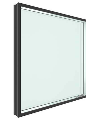
GL01 a. MATERIAL TYPE: INSULATED COATED GLASS VISION b. OVERALL THICKNESS: 1 IN NOMINAL c. AIR SPACE: 1/2"; ALUMINUM BLACK ARGON d. INBOARD LINTEL: CLEAR HS. 1 1/4" THICK GLASS e. BASIS OF DESIGN 1" INSULATED LOW-E GLASS
