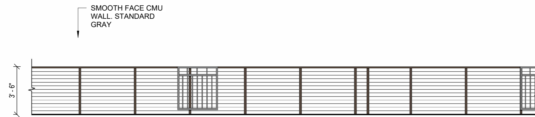
5 NORTH PATIO FENCE ELEVATION 1/4" = 1'-0"
