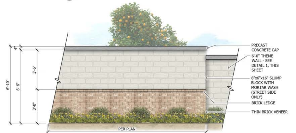
3 2'-0" View Fence over 4'-0" CMU Wall SCALE: 1/2"=1'-0"
