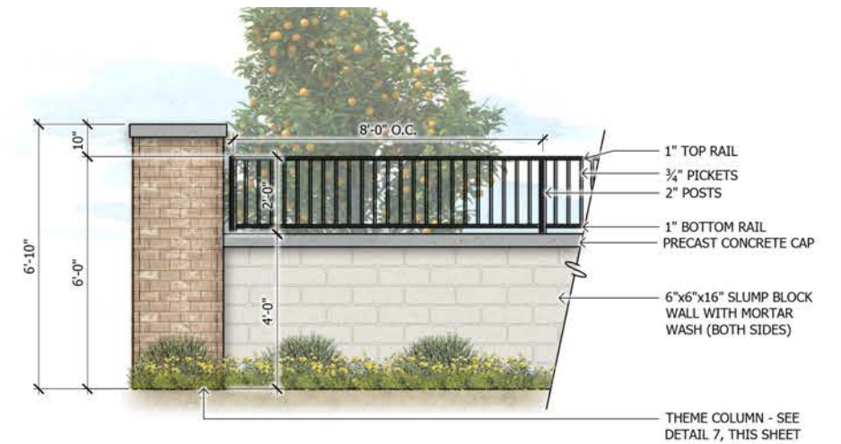
3 2'-0" View Fence over 4'-0" CMU Wall SCALE: 1/2"=1'-0"
