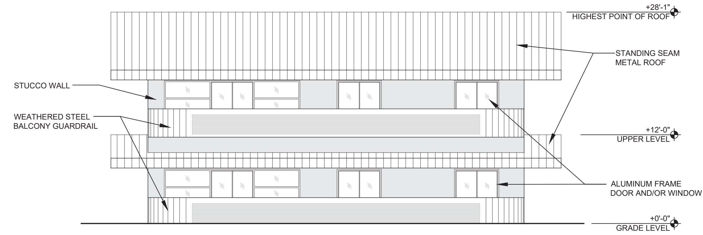
TYP TWO LEVEL REAR BLDG ELEV
