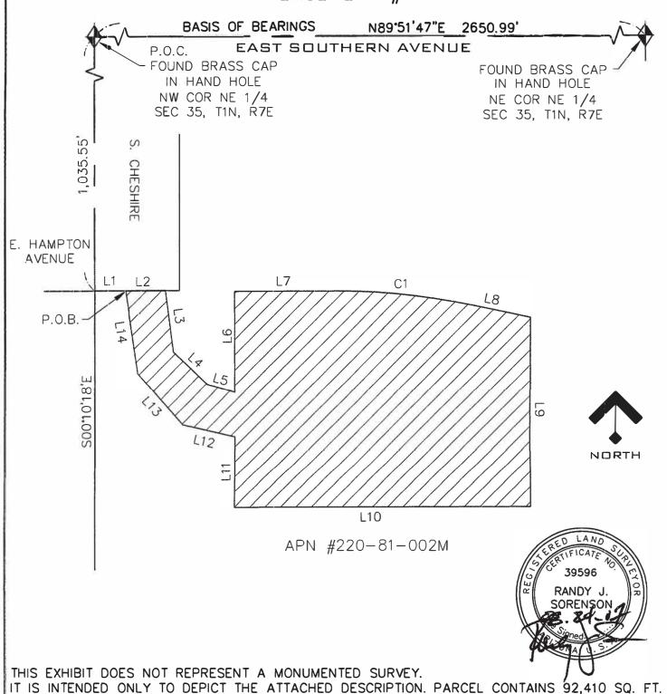
A TEMPORARY DRAINAGE EASEMENT #4 WITHIN THE NORTHEAST QUARTER OF SECTION 35, T1N, R7E, GILA & SALT RIVER MERIDIAN, MARICOPA COUNTY, ARIZONA.
