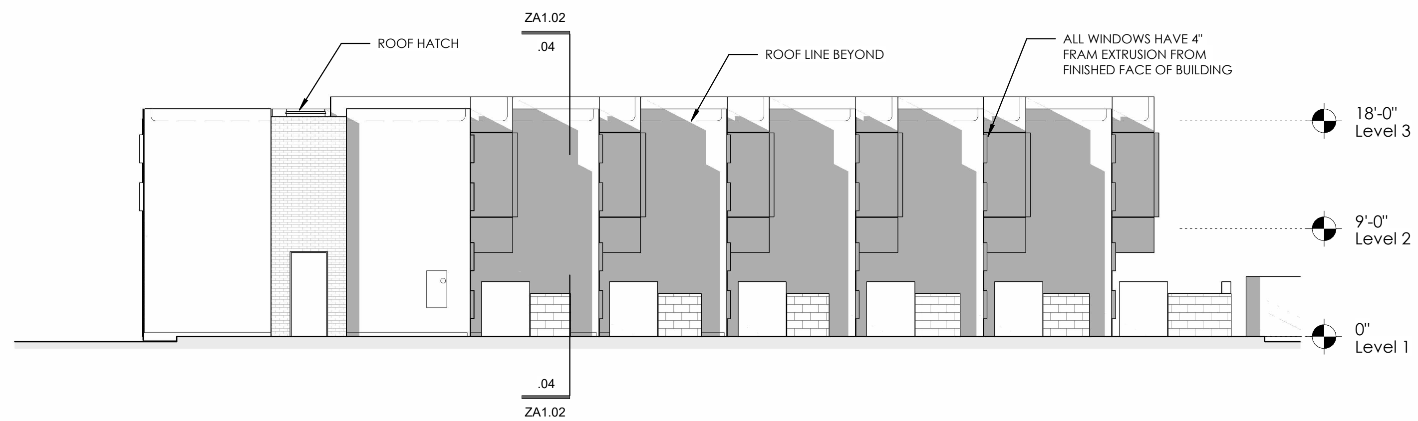
Building Type 'A' South Elevation .01 1/8" = 1'-0"
