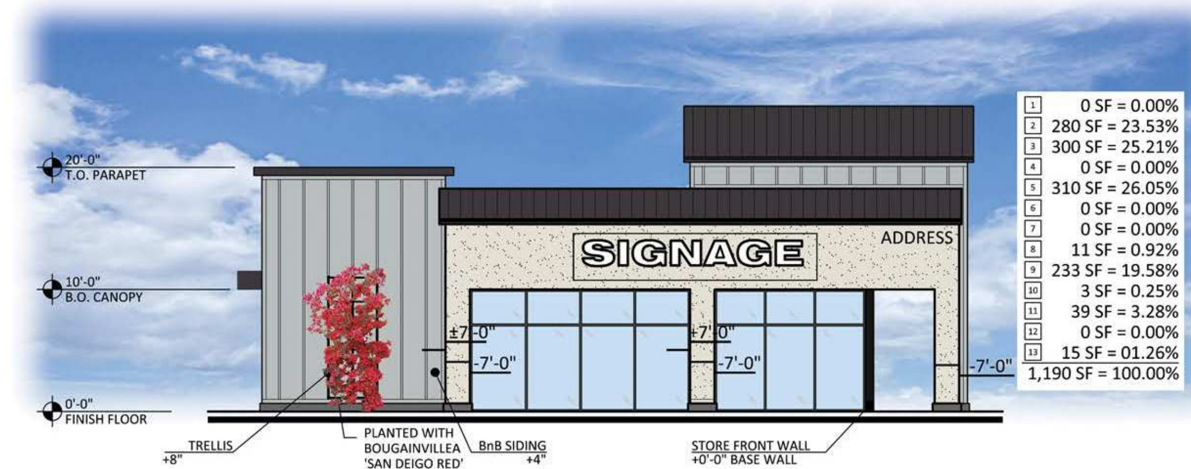
3 WEST ELEVATION PLAN SCALE: 1/8" = 1'-0"
