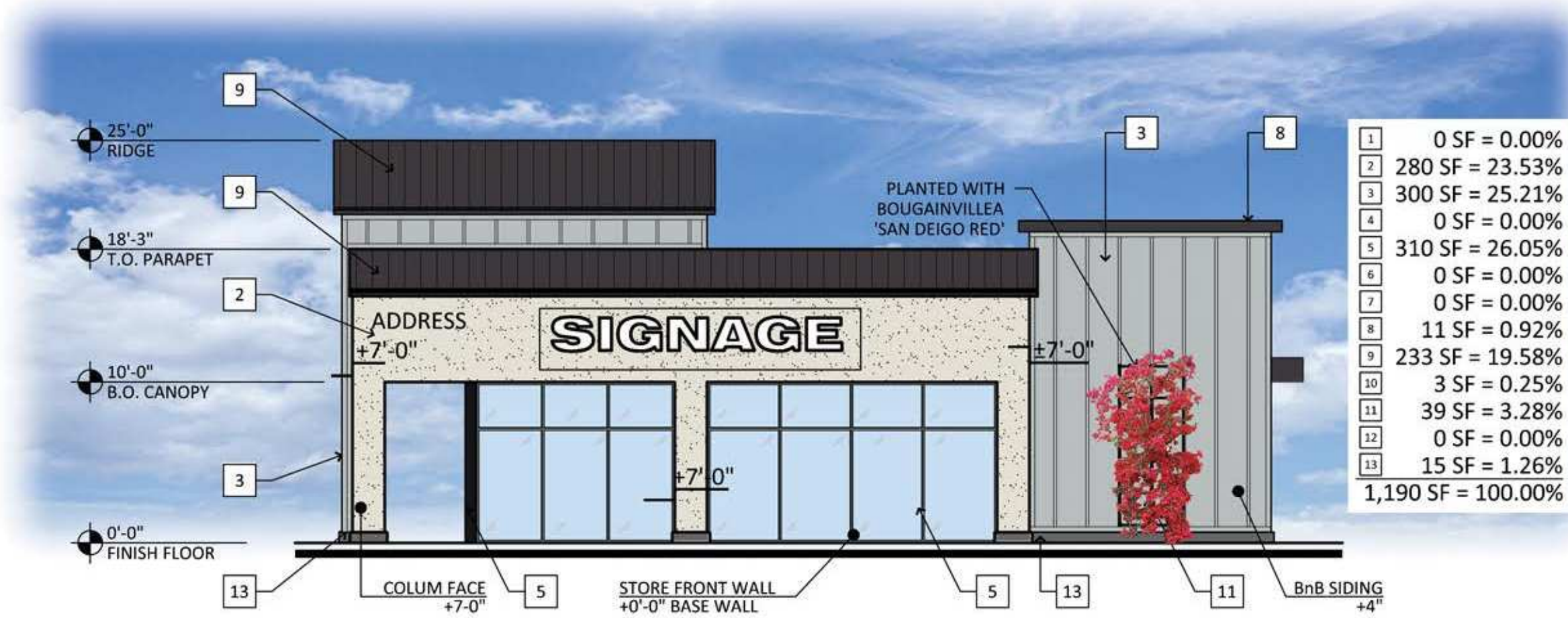
2 EAST ELEVATION PLAN SCALE: 1/8" = 1'-0"
