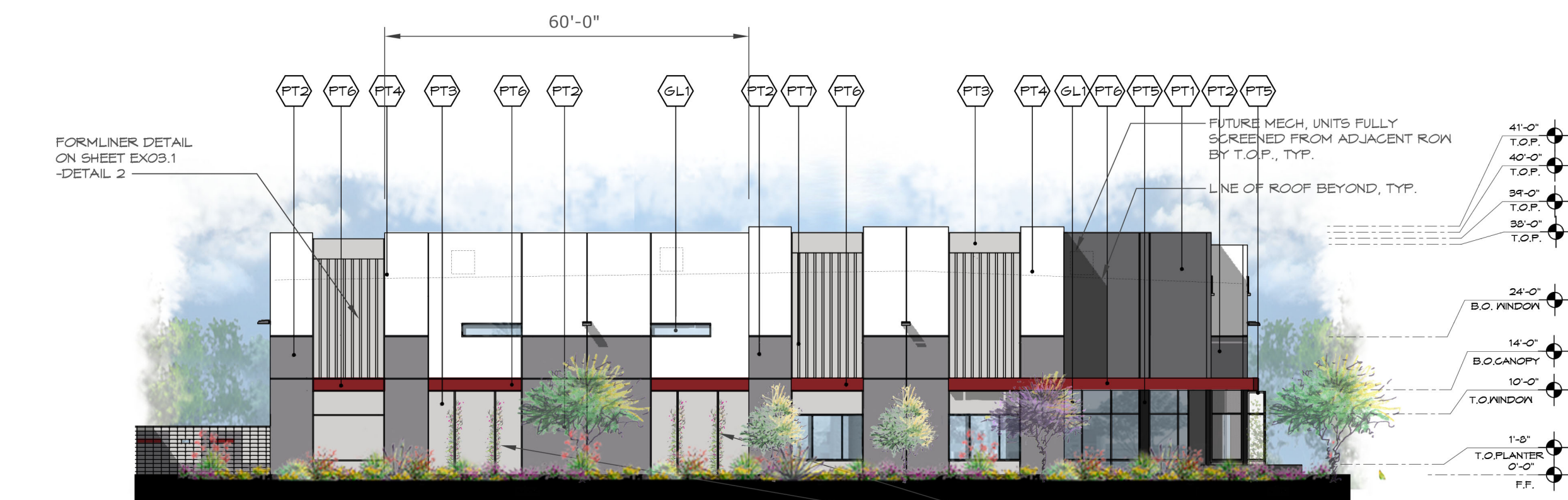
2 SOUTH ELEVATION - BUILDING B Scale: 1" = 20'
