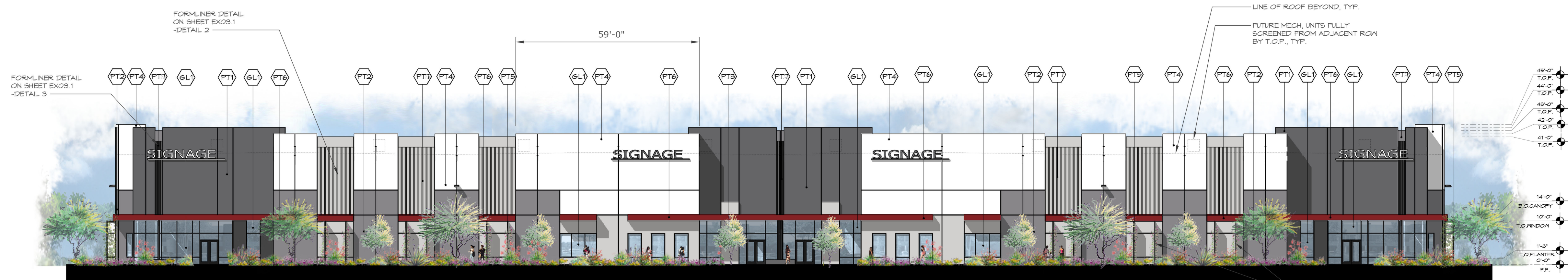
1 SOUTH ELEVATION - BUILDING C Scale: 1" = 20'
