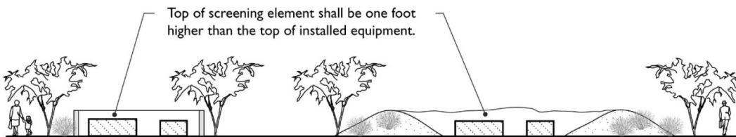
FIGURE 11-30-9.A.(2): SCREENING OF GROUND-MOUNTED EQUIPMENT
