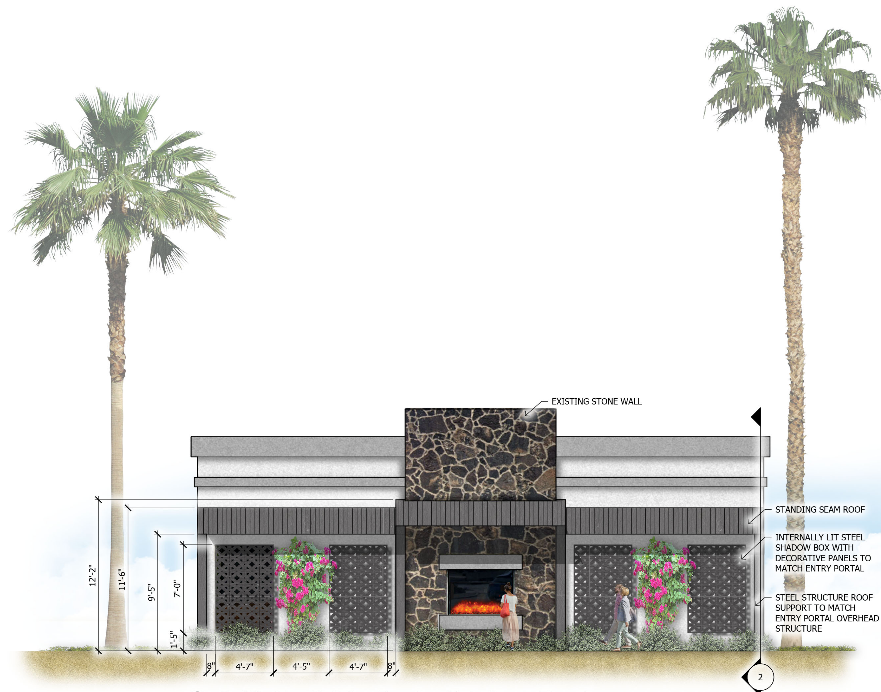
1 Co-Working Building Facade - Main Street Elevation SCALE: 1/4"=1'-0"
