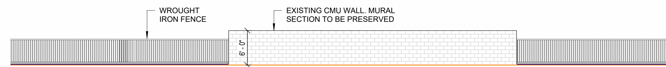
4 SOUTH FENCING ELEVATION 1" = 10'-0"
