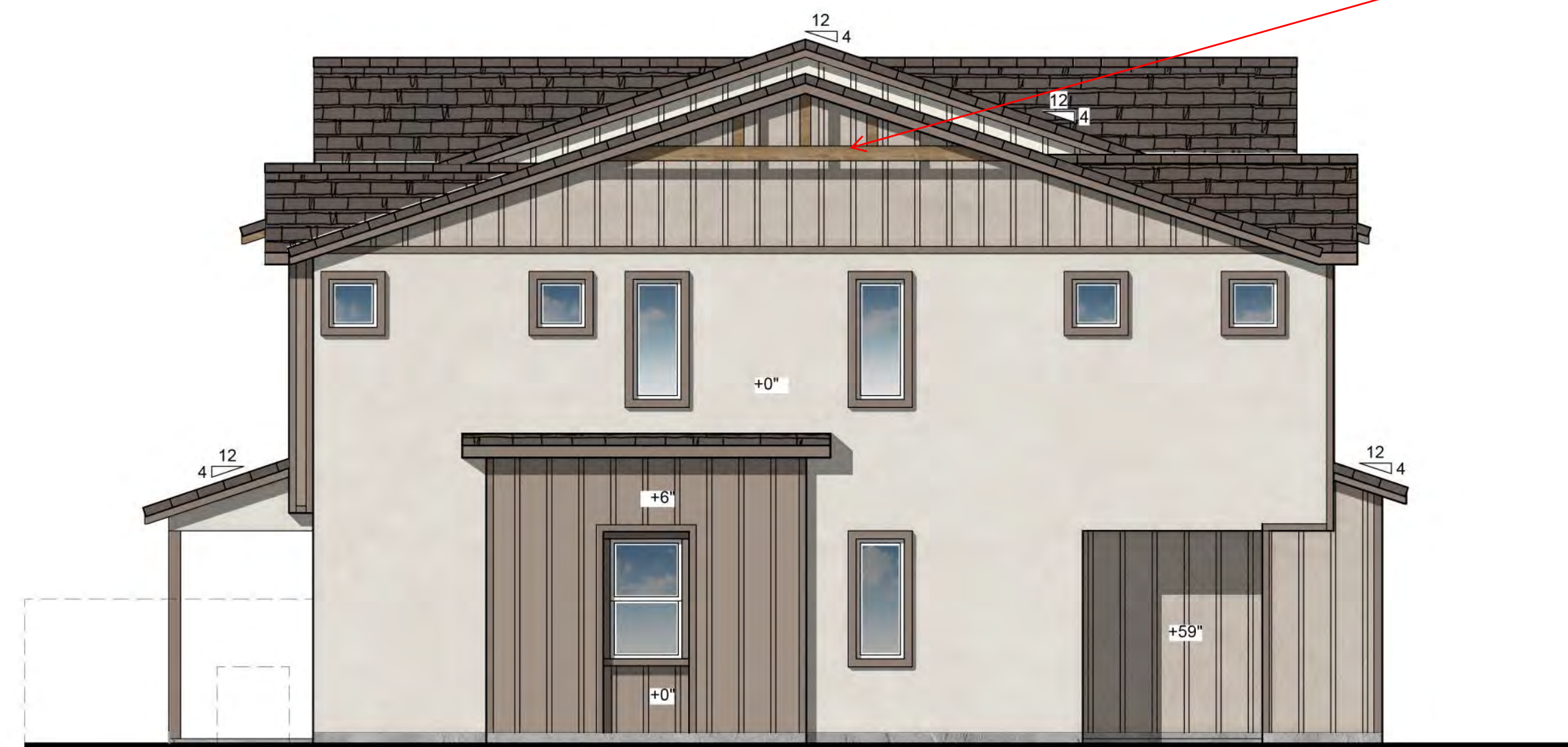
LEFT ELEVATION 6-PLEX MODERN FARMHOUSE 3/16" = 1'-0"
