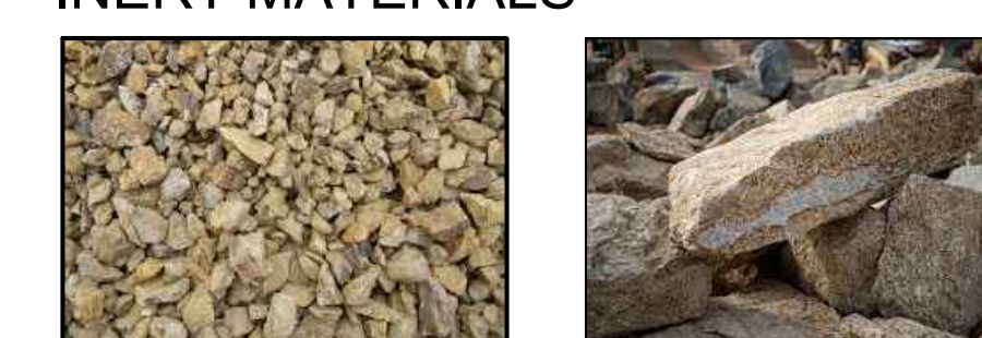
DECOMPOSED GRANITE MADISON DESERT GOLD 1/2" SCREENED, 2" DEPTH, MIN. BOULDER MADISON DESERT GOLD LARGE 3x3x2'
