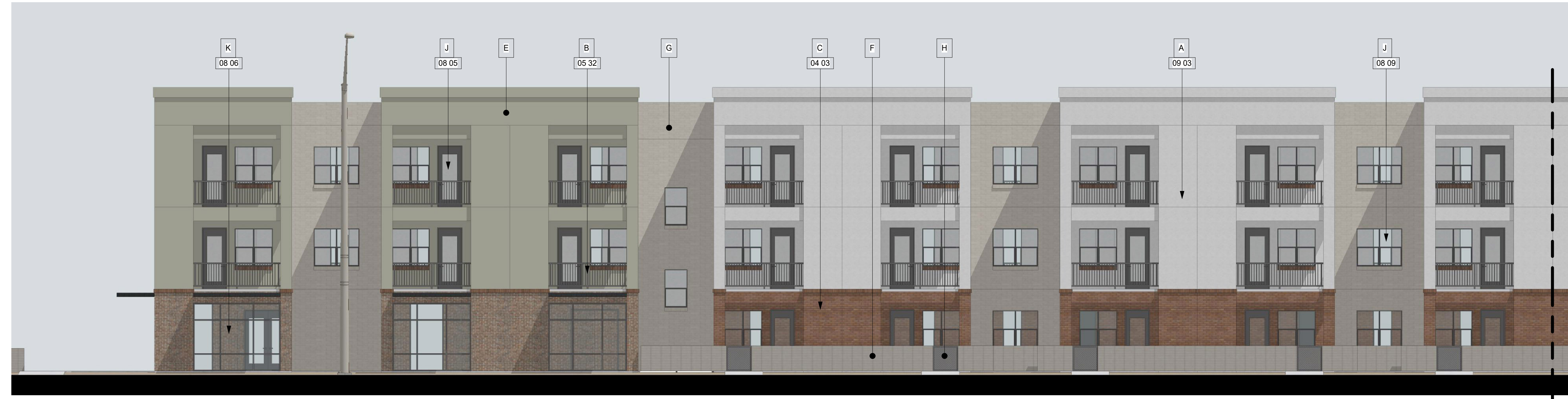
1 SOUTH COLORED ELEVATION - BLDG 1 AREA 1B 1/8" = 1'-0"
