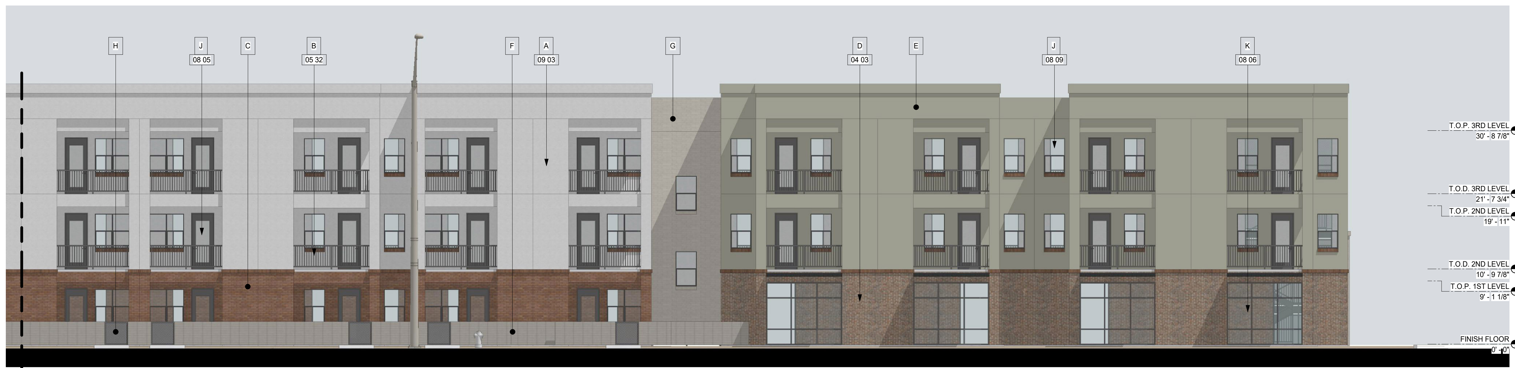
2 SOUTH COLORED ELEVATION - BLDG 1 AREA 1A 1/8" = 1'-0"
