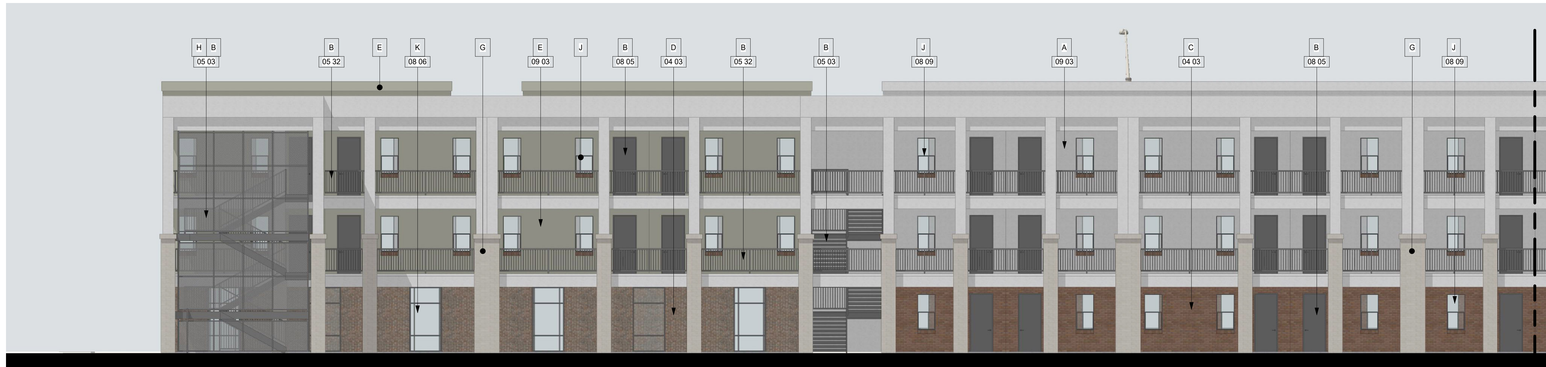
2 NORTH COLORED ELEVATION - BLDG 1 AREA 1A 1/8" = 1'-0"
