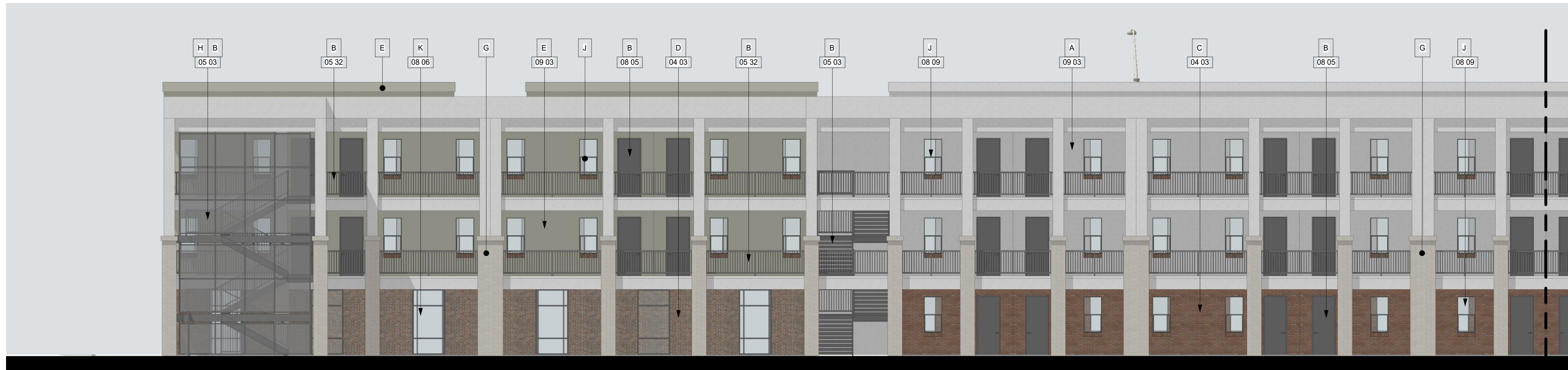
2 NORTH COLORED ELEVATION - BLDG 1 AREA 1A 1/8" = 1'-0"
