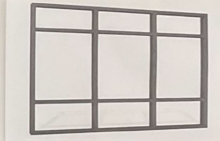
STOREFRONT GLAZING CLEAR LOW-E GLAZING
