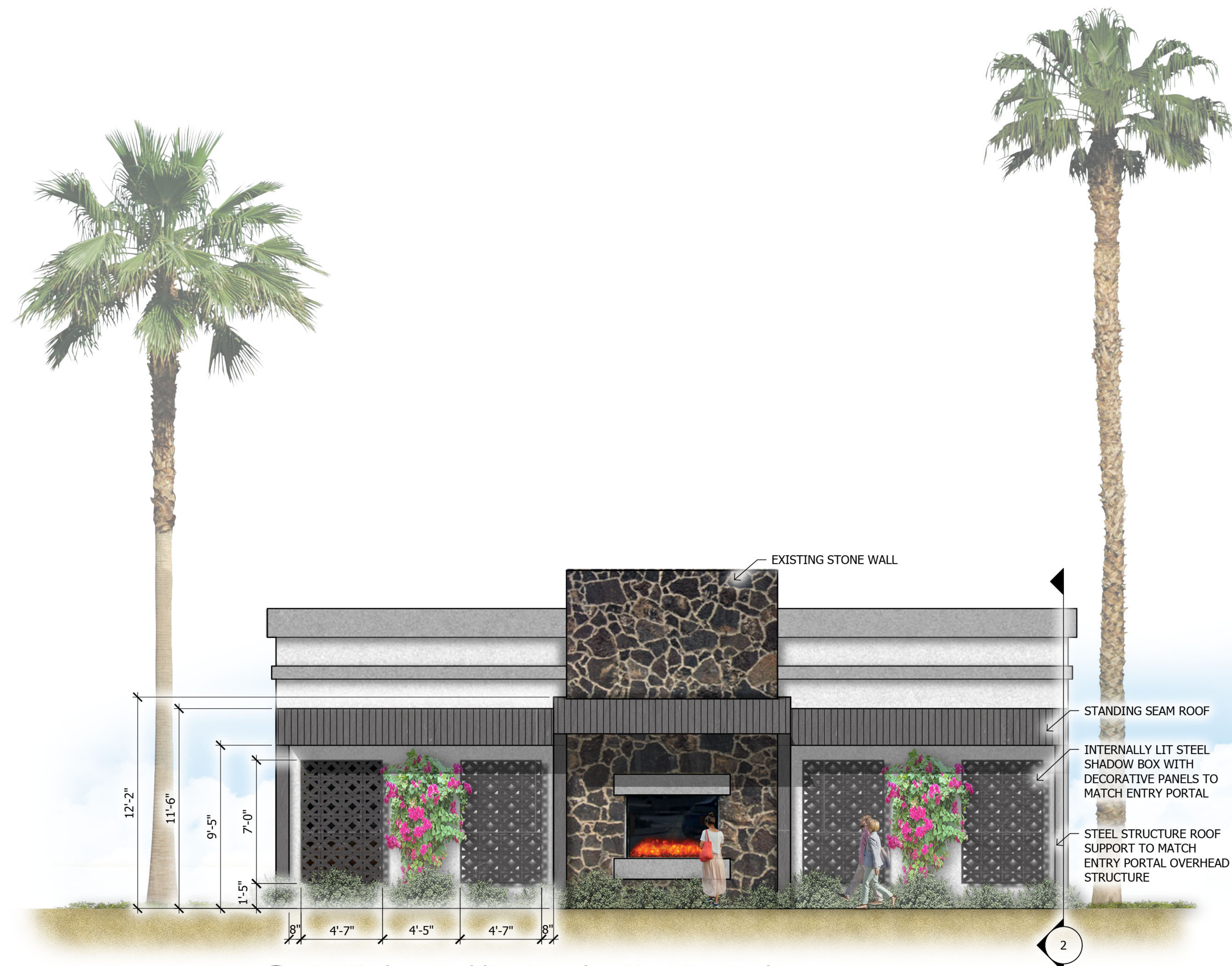
1 Co-Working Building Facade - Main Street Elevation SCALE: 1/4"=1'-0"
