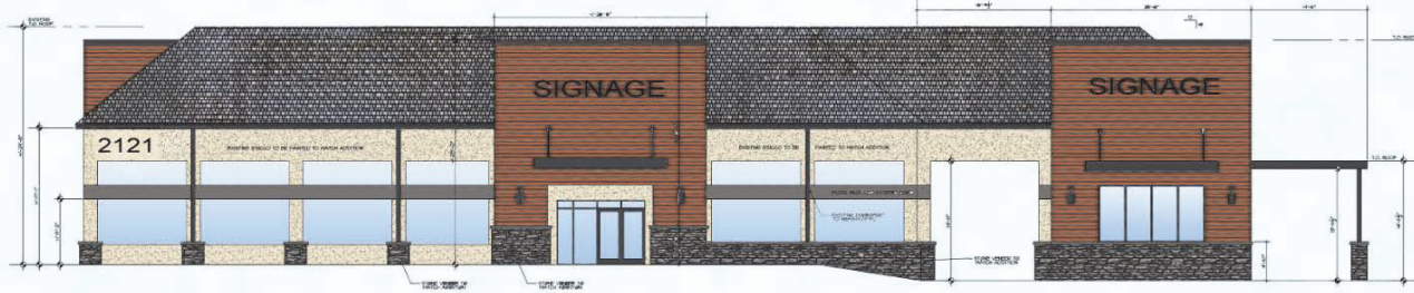
PROPOSED WEST ELEVATION KIONA AVE VIEW 1/8"=1'-0"
