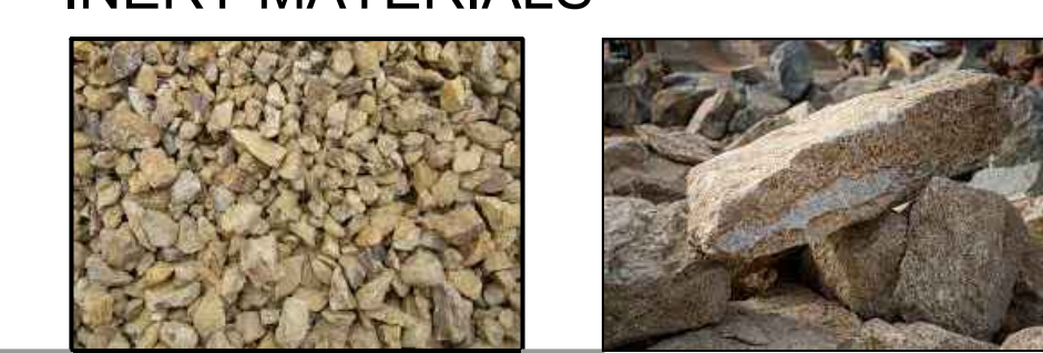
DECOMPOSED GRANITE MADISON DESERT GOLD 1/2" SCREENED, 2" DEPTH, MIN. BOULDER MADISON DESERT GOLD LARGE 3x3x2'
