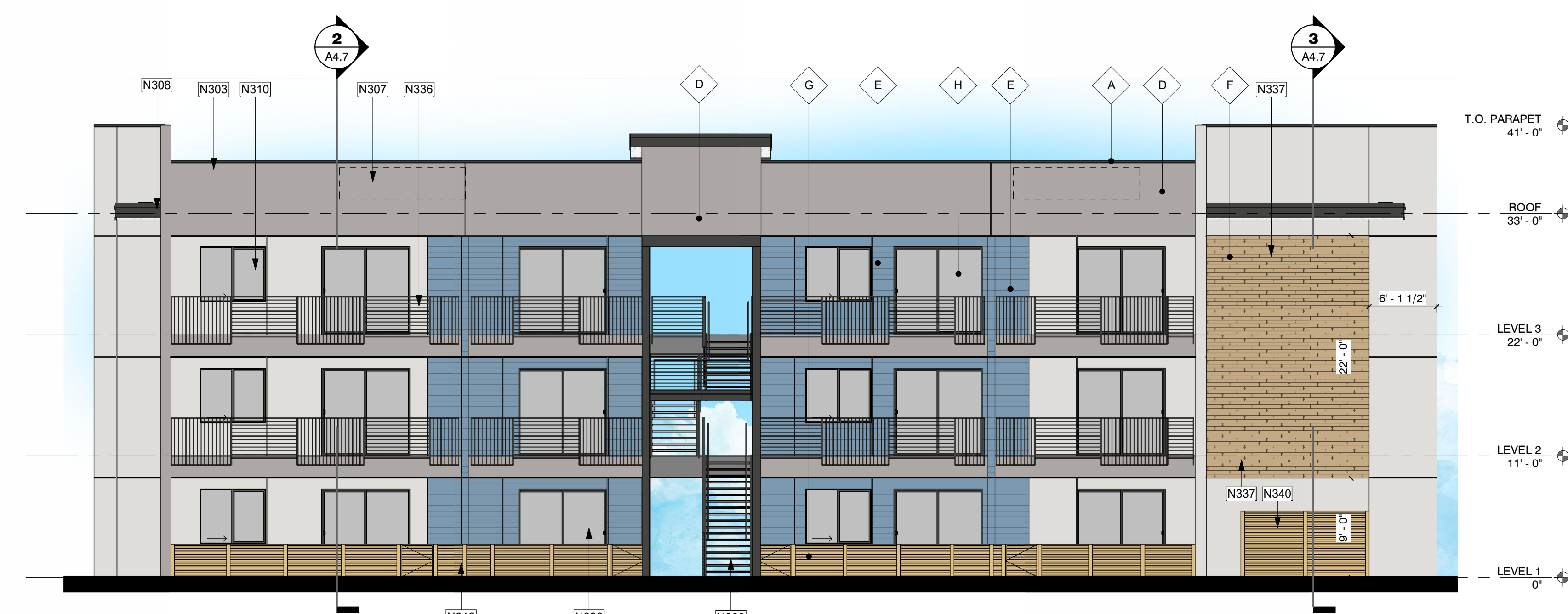
2 Building Type 3 - Elevation 2 1/8" = 1'-0"
