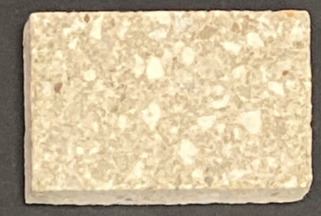
B-4 - 8x8x16 GROUND FACE CONCRETE MASONRY UNIT RUNNING BOND MANUF: ECHELON MASONRY - TRENDSTONE COLOR: MISSION WHITE
