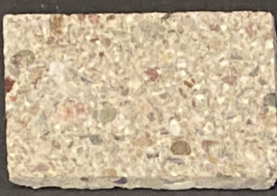
B-1 - 4x4x8 GROUND FACE CONCRETE MASONRY UNIT STACK BOND MANUF: ECHELON MASONRY - TRENDSTONE COLOR: PEBBLE BEACH
