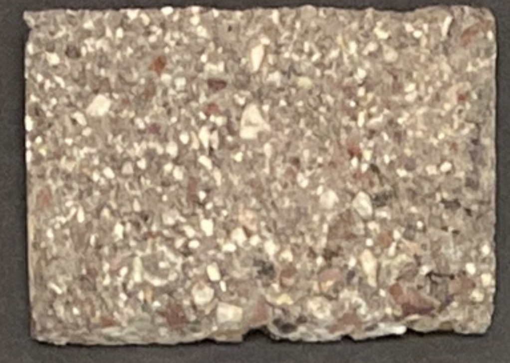
B-2 - 4x4x8 TEXTURED CONCRETE MASONRY UNIT STACK BOND MANUF: ECHELON MASONRY - MESASTONE COLOR: BLACK MOUNTAIN
