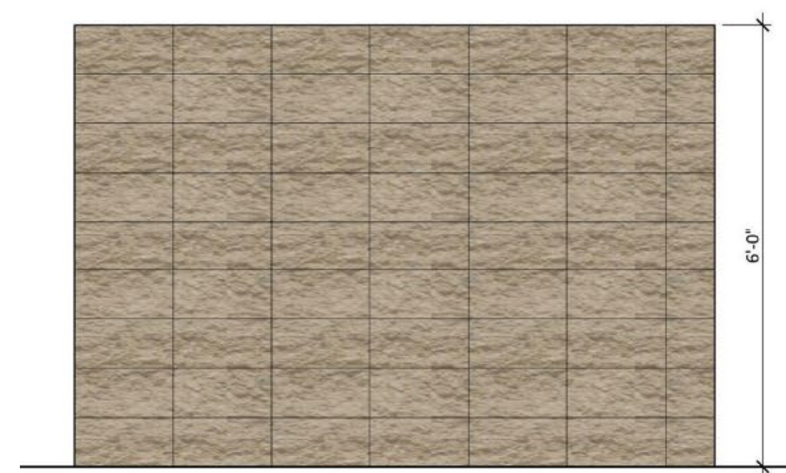
4 STACKED CMU WALL AT 6'-0" TRANSFORMER SCREEN 1/16" = 1'-0" P-HI1-07
