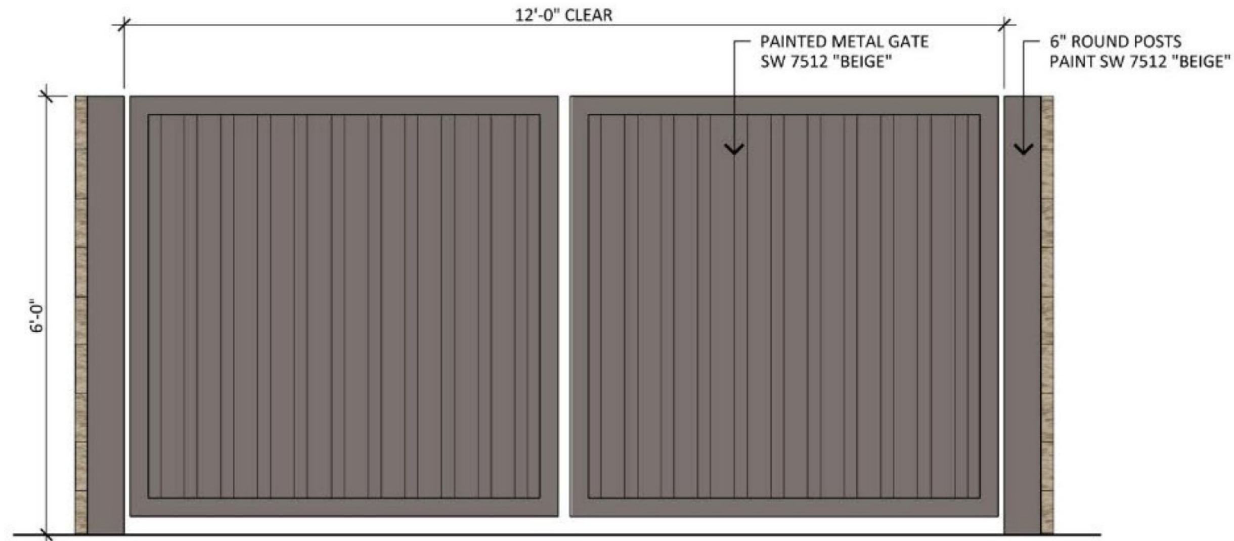
2 TRASH ENCLOSURE GATE 1/16" = 1'-0" P-HI1-02
