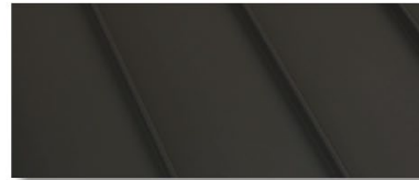
STANDING SEAM METAL ROOF COATED METALS GROUP - DARK BRONZE | STANDING SEAMS AT 16" O.C. | SMOOTH FINISH
