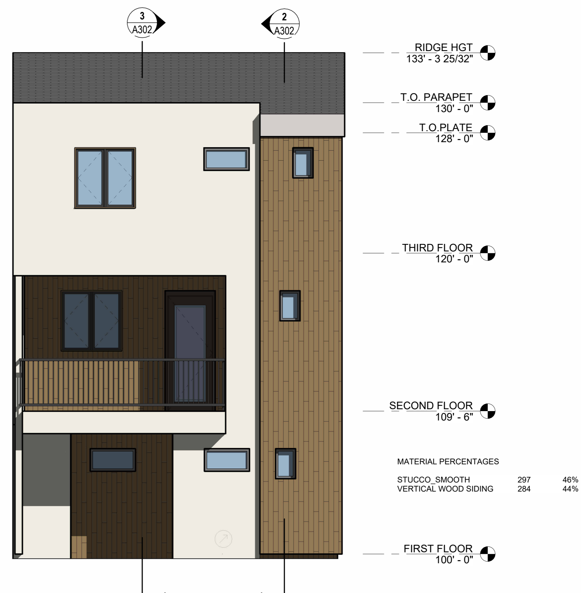
② UNIT C, ENTRY ELEVATION 1/4" = 1'-0"
