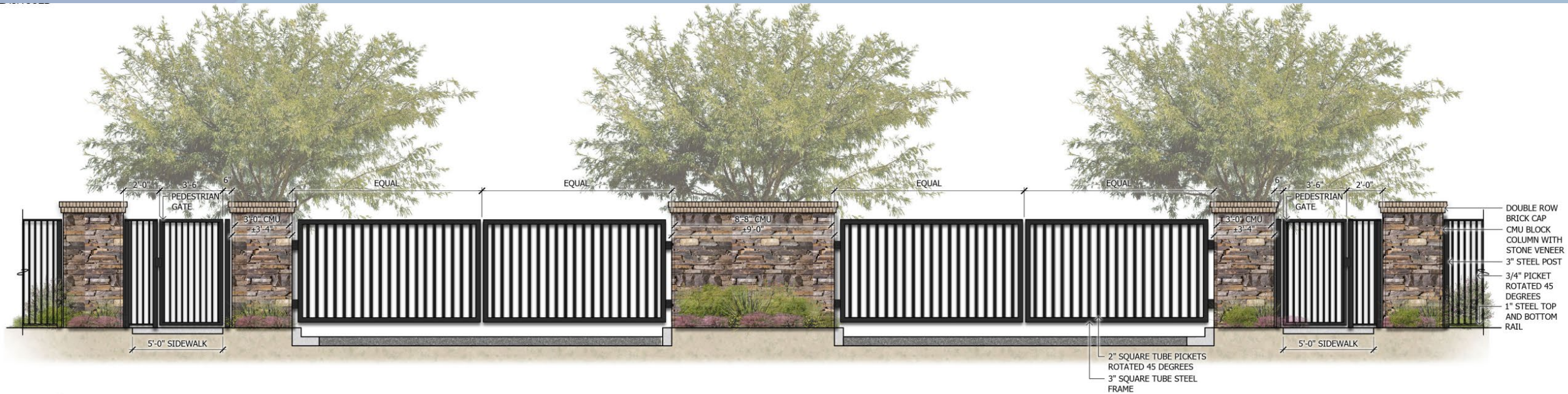
1 Vehicular Access Gate SCALE: 3/8"=1'-0"
