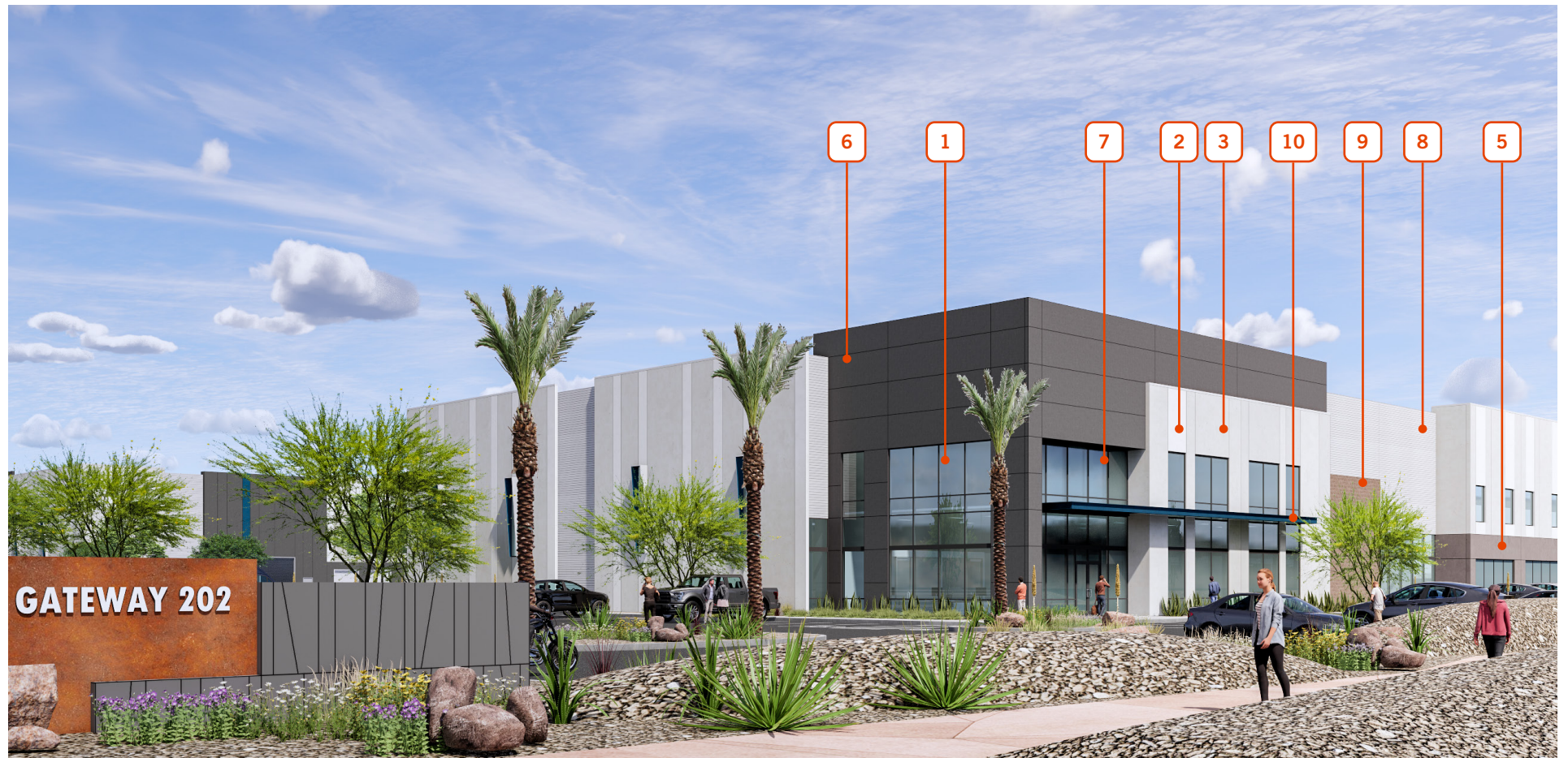
9 CMU BLOCK: COLOR/FINISH: MERLOT / SPLIT FACE (OR APPROVED EQUIVALENT MATERIAL WITH COMPARABLE COLOR AND TEXTURE, SUCH AS FORMLINER)
