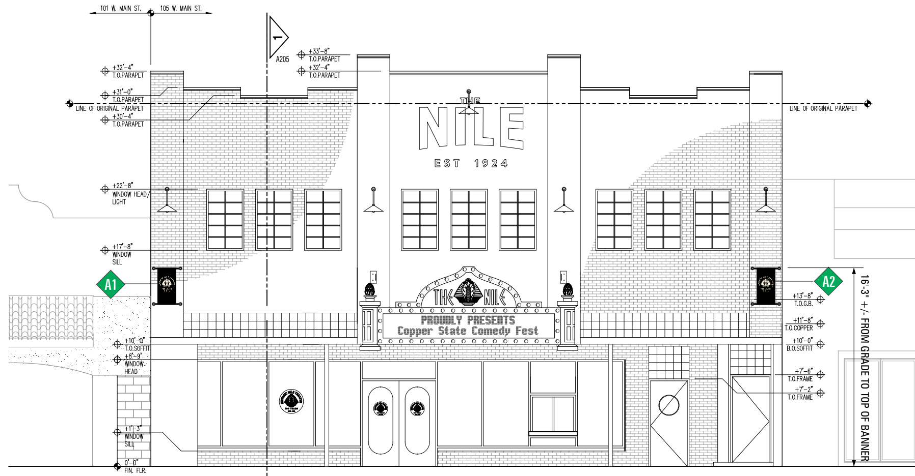
NORTH ELEVATION - EXISTING BANNER SIGNAGE SCALE: 1/8" = 1'-0"
