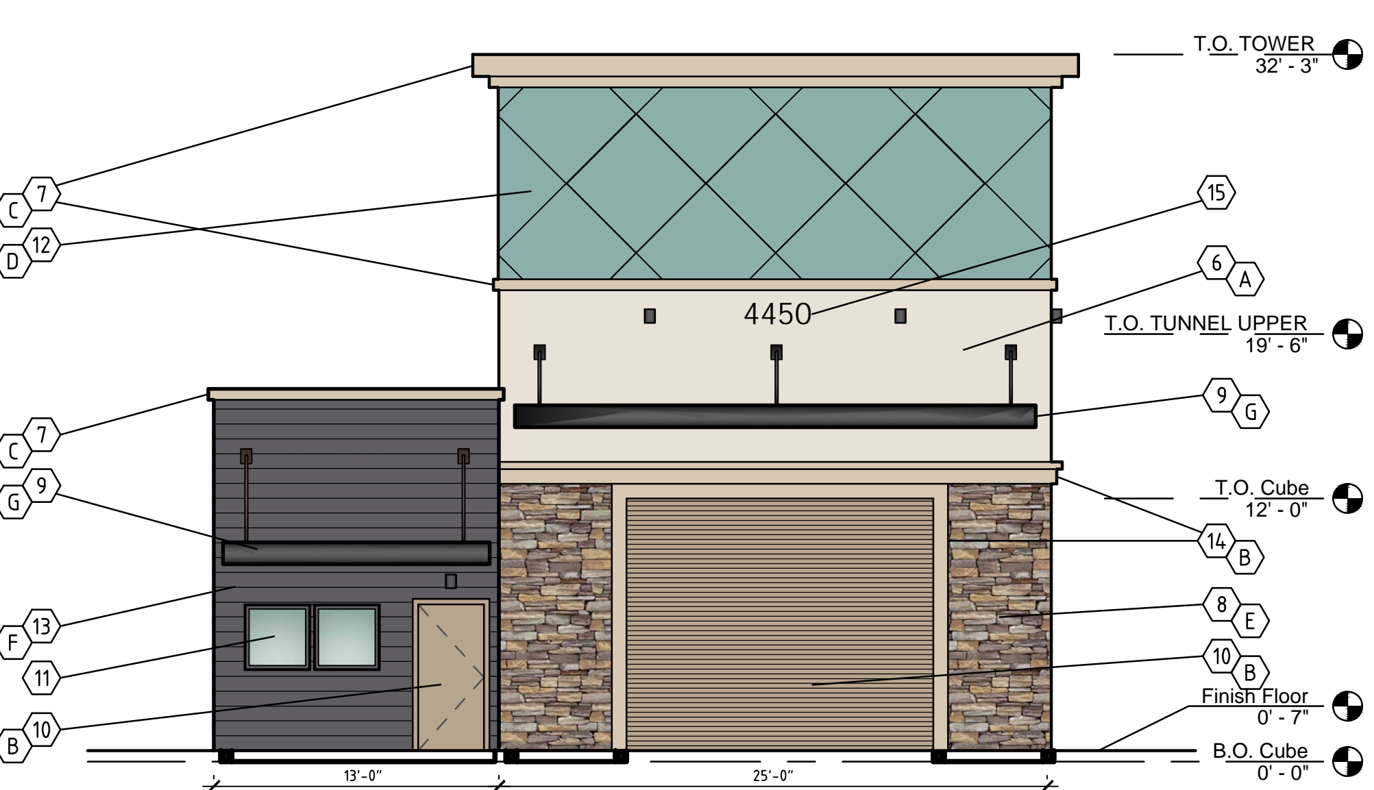
B EXTERIOR ELEVATION - FRONT - SOUTHEAST 3/16 = 1' - 0"
