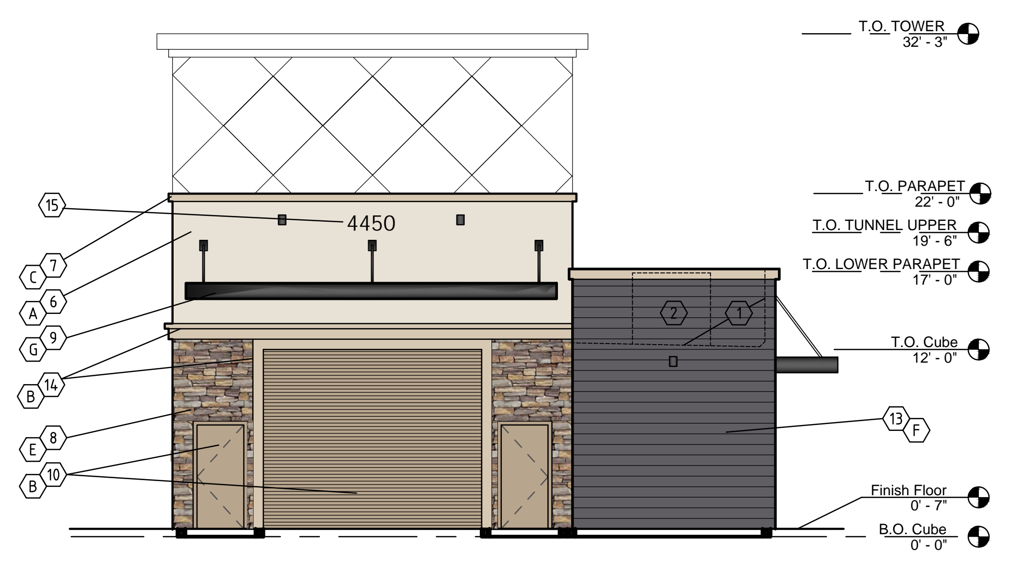
D EXTERIOR ELEVATION - REAR - NORTHWEST 3/16 = 1' - 0"
