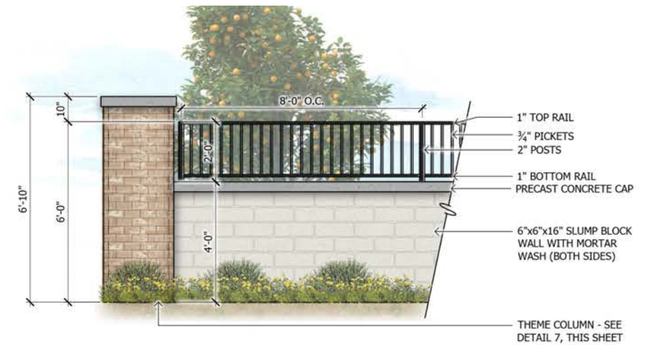
3 2'-0" View Fence over 4'-0" CMU Wall SCALE: 1/2"=1'-0"
