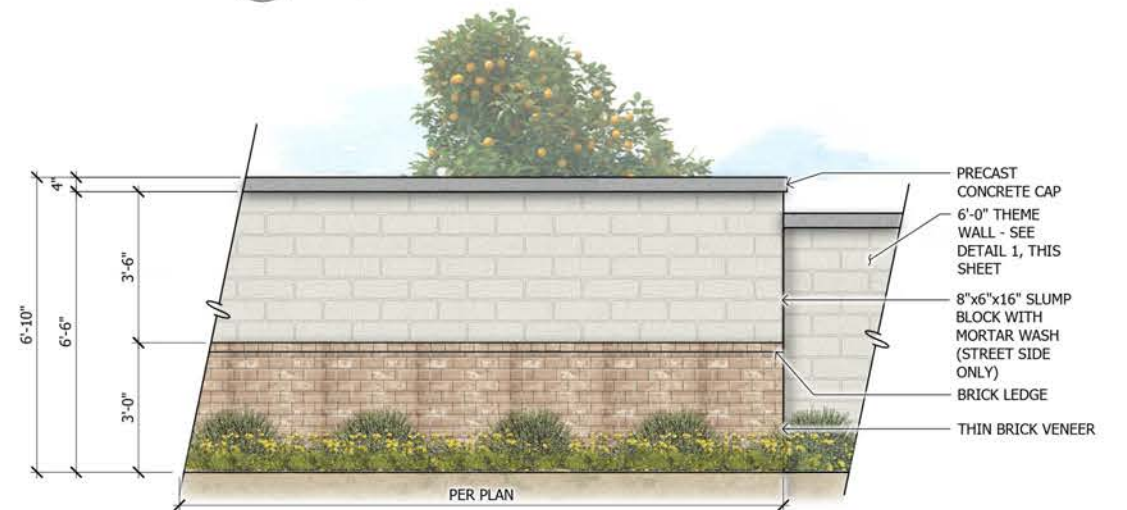
3 2'-0" View Fence over 4'-0" CMU Wall SCALE: 1/2"=1'-0"
