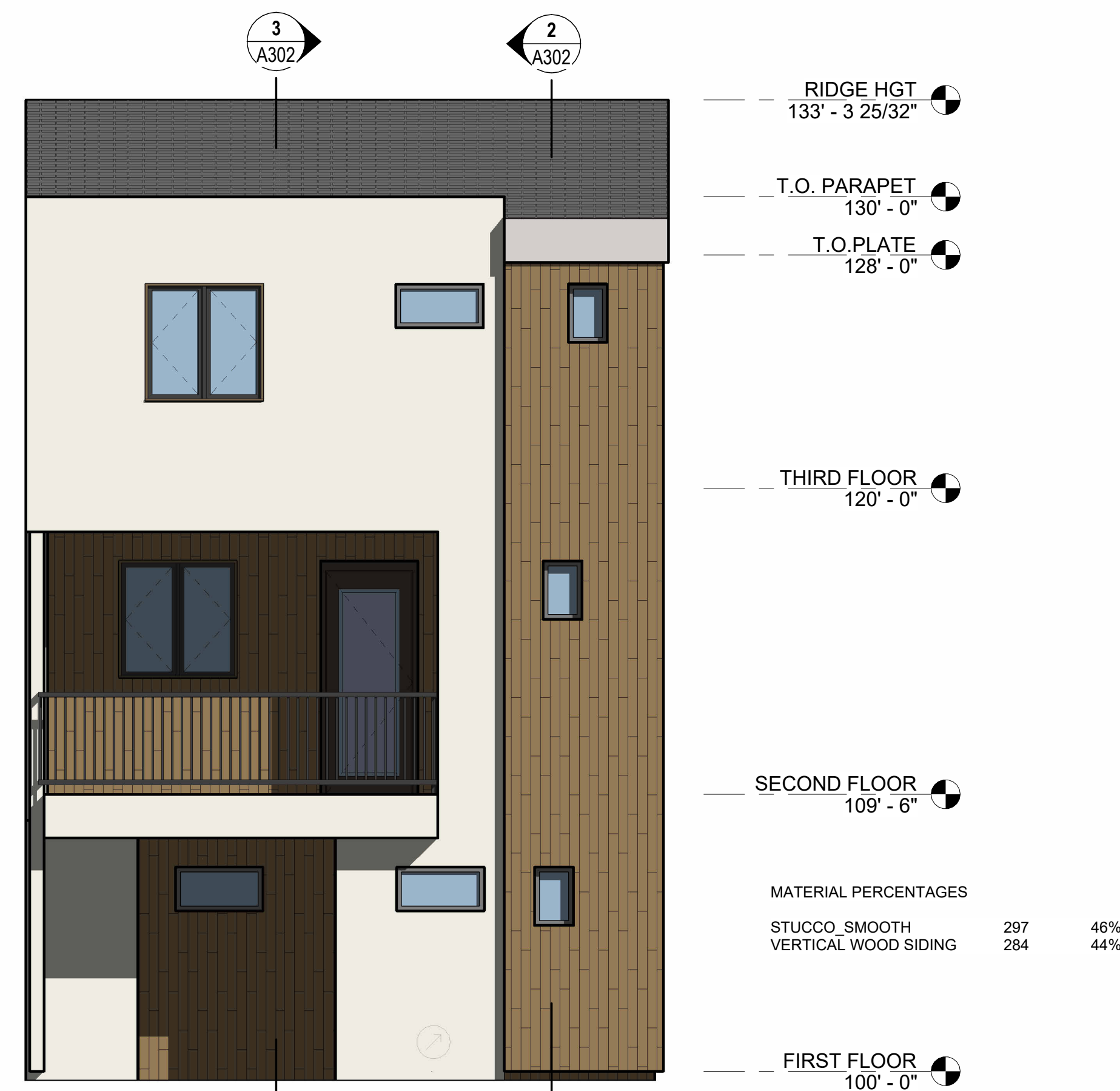
② UNIT C ENTRY ELEVATION 1/4" = 1'-0"
