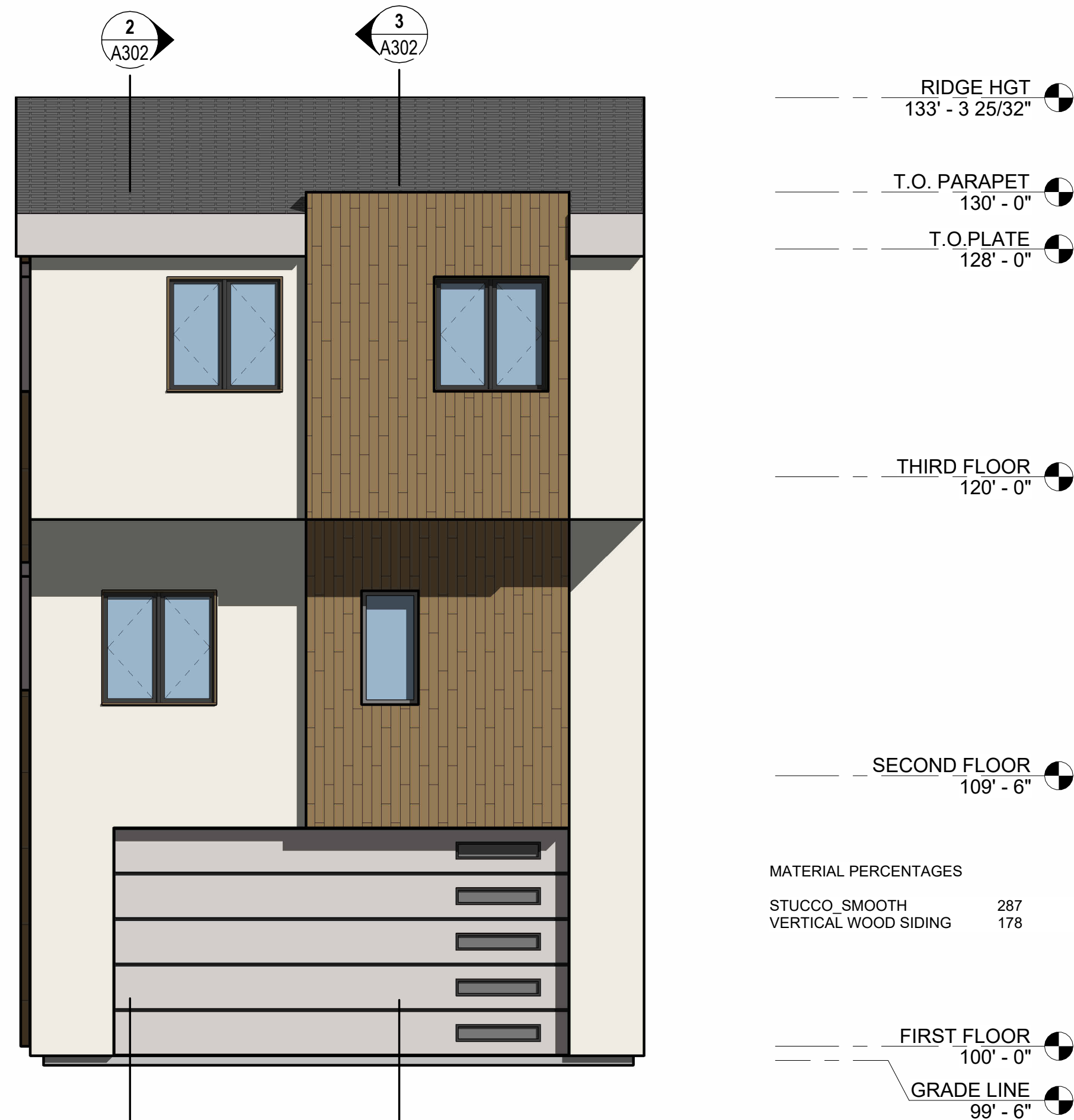
③ UNIT C GARAGE ELEVATION 1/4" = 1'-0"
