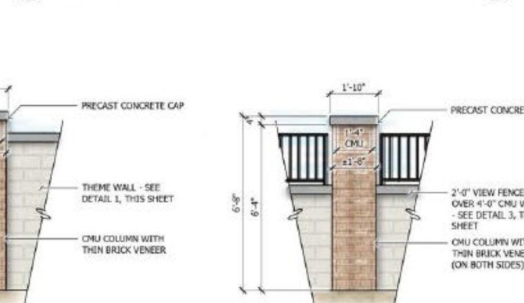
8 Intermediate Wall Column SCALE: 1/2"=1'-0"
