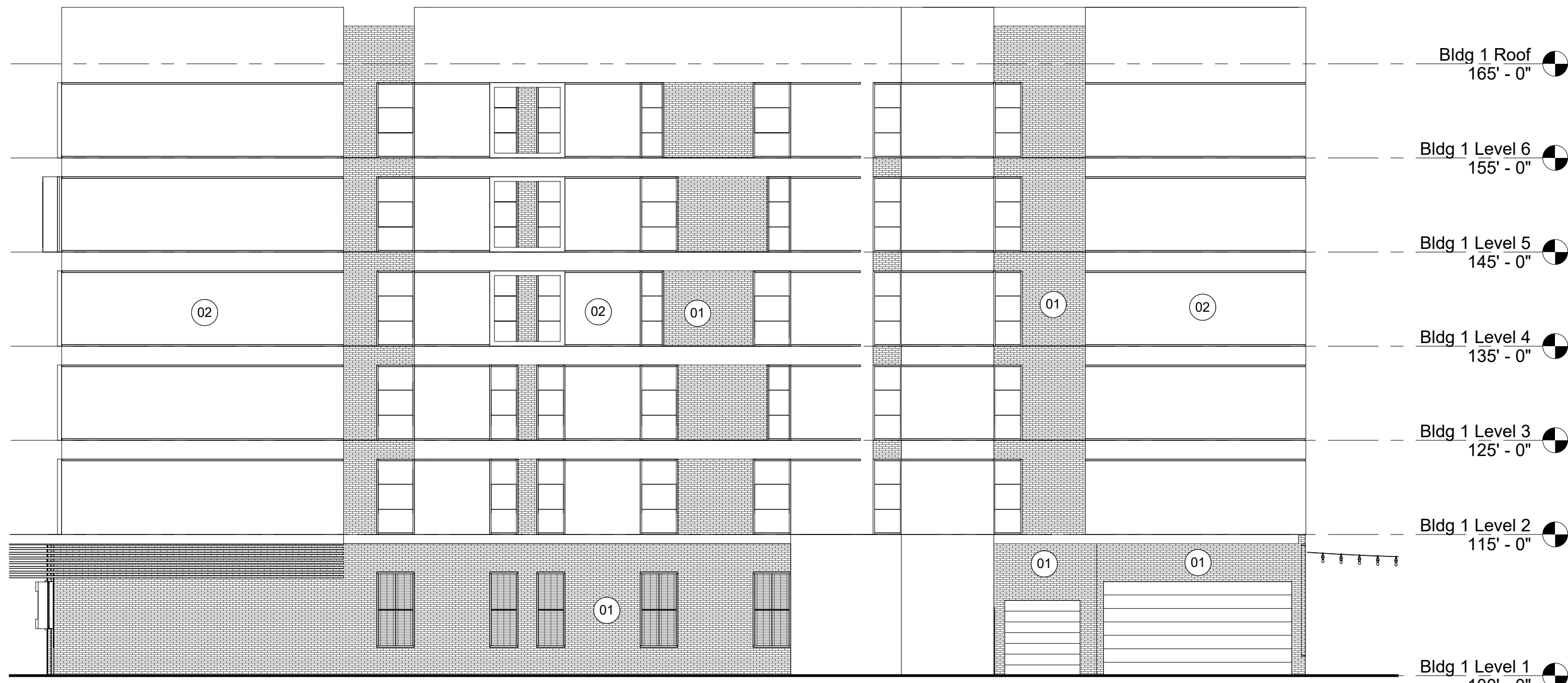
3 BLDG 1 SOUTH ELEVATION 3/32" = 1'-0"
