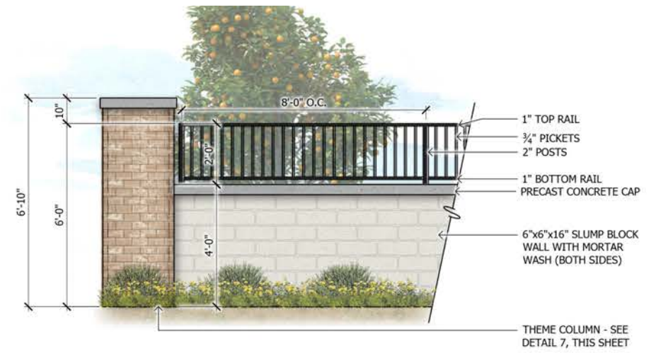
3 2'-0" View Fence over 4'-0" CMU Wall SCALE: 1/2"=1'-0"
