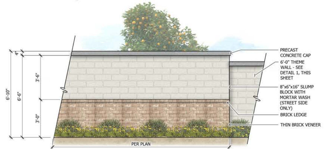
3 2'-0" View Fence over 4'-0" CMU Wall SCALE: 1/2"=1'-0"
