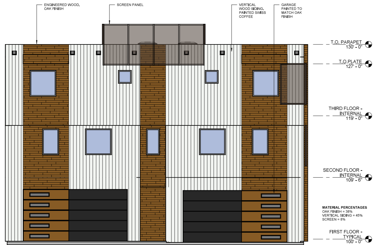
③ GARAGE ELEVATION 1/4" = 1'-0"
