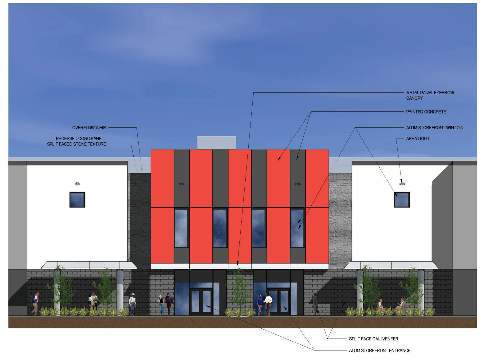
NORTH ELEVATION DETAIL - PECOS ROAD FRONTAGE 1/8" = 1'-0"
