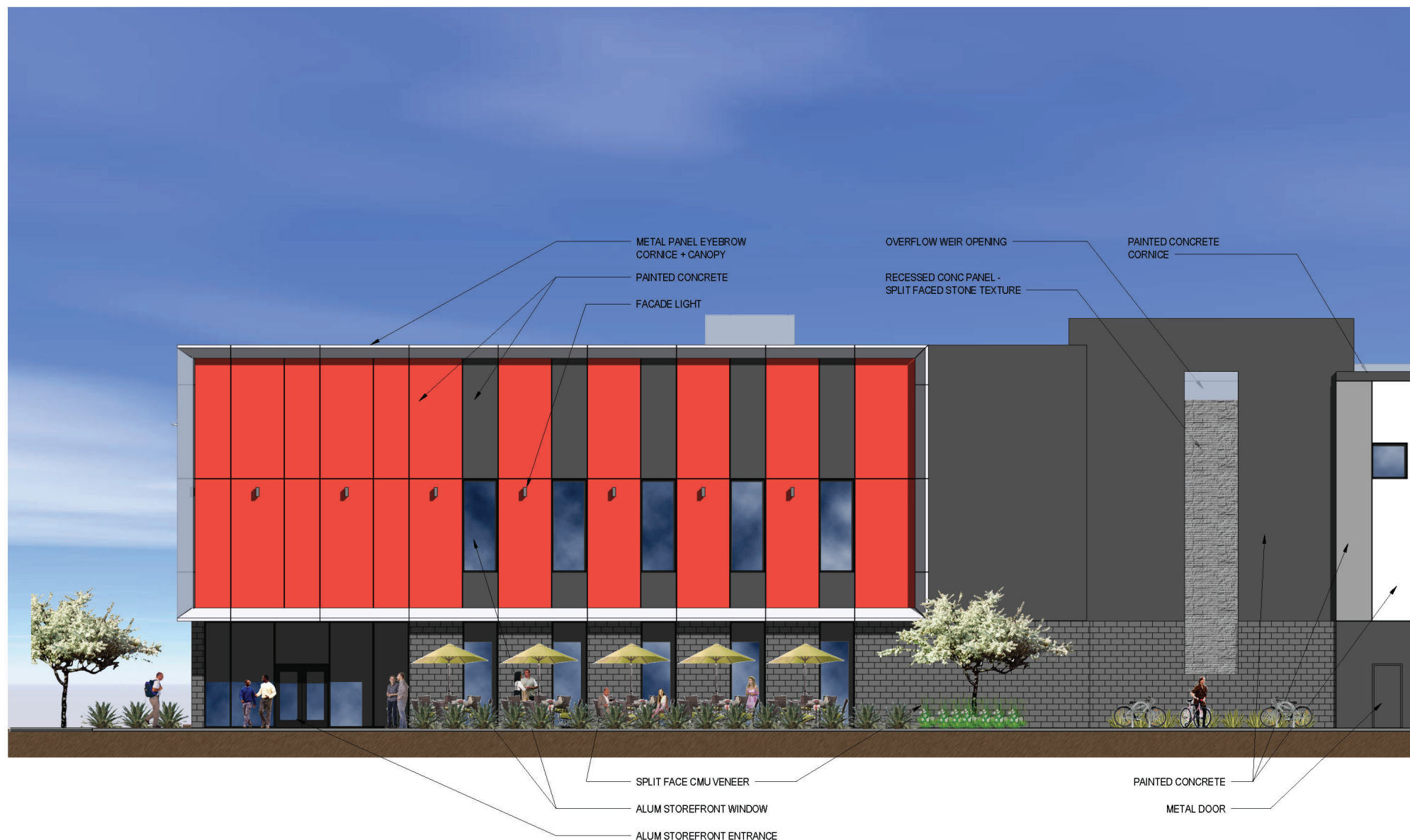
NORTH ELEVATION DETAIL - PECOS ROAD FRONTAGE 1/8" = 1'-0"
