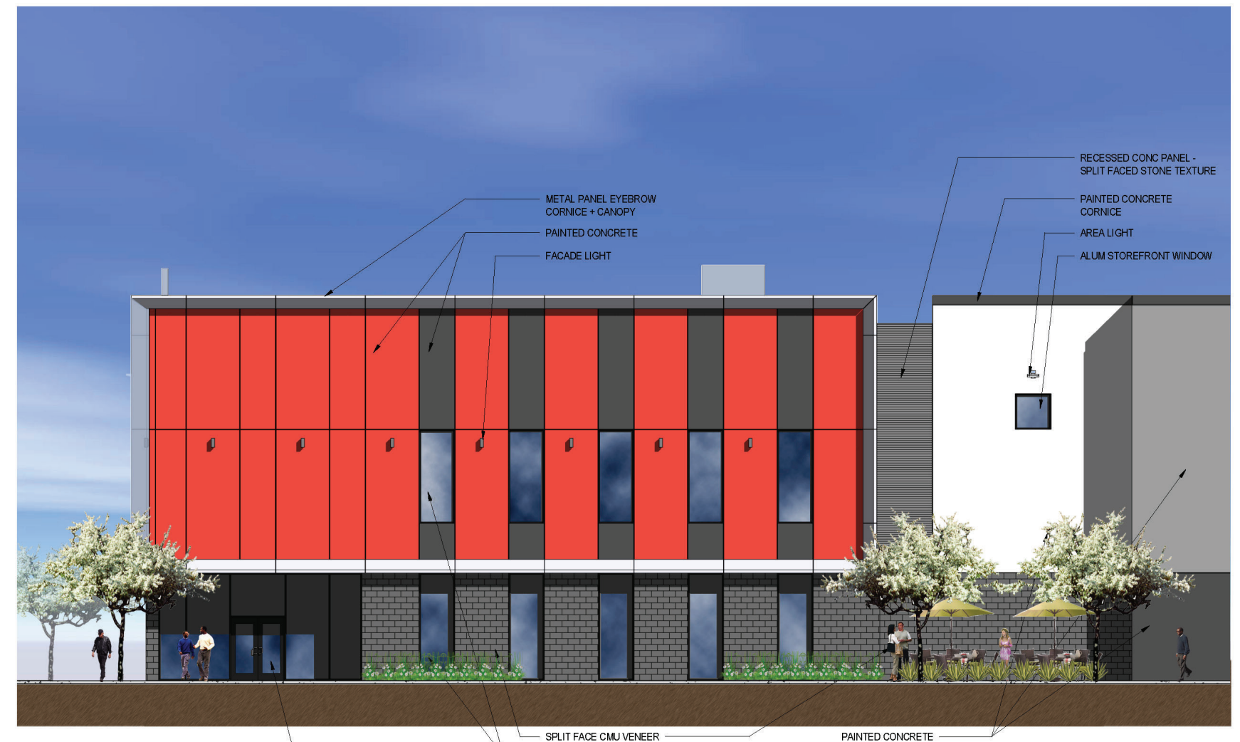
WEST ELEVATION DETAIL - CRISMON ROAD FRONTAGE 1/8" = 1'-0"
