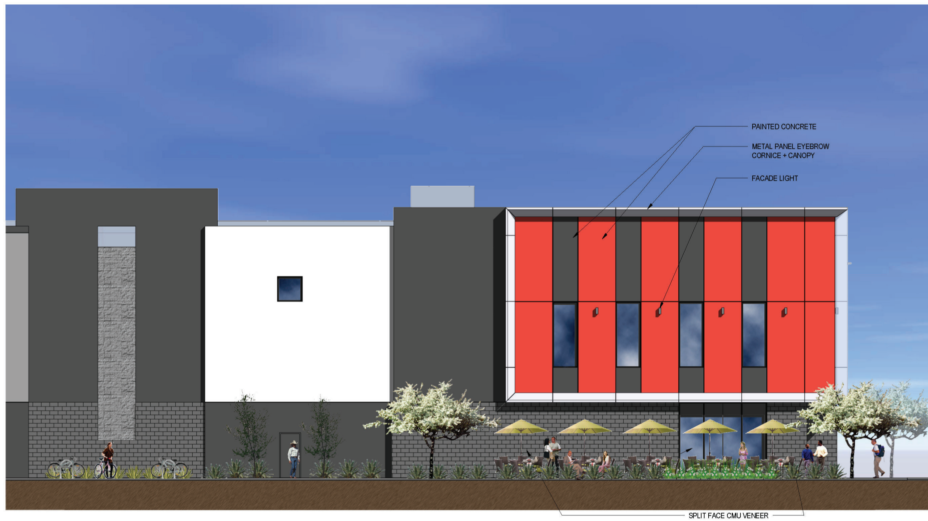
NORTH ELEVATION DETAIL - PECOS ROAD FRONTAGE 1/8" = 1'-0"
