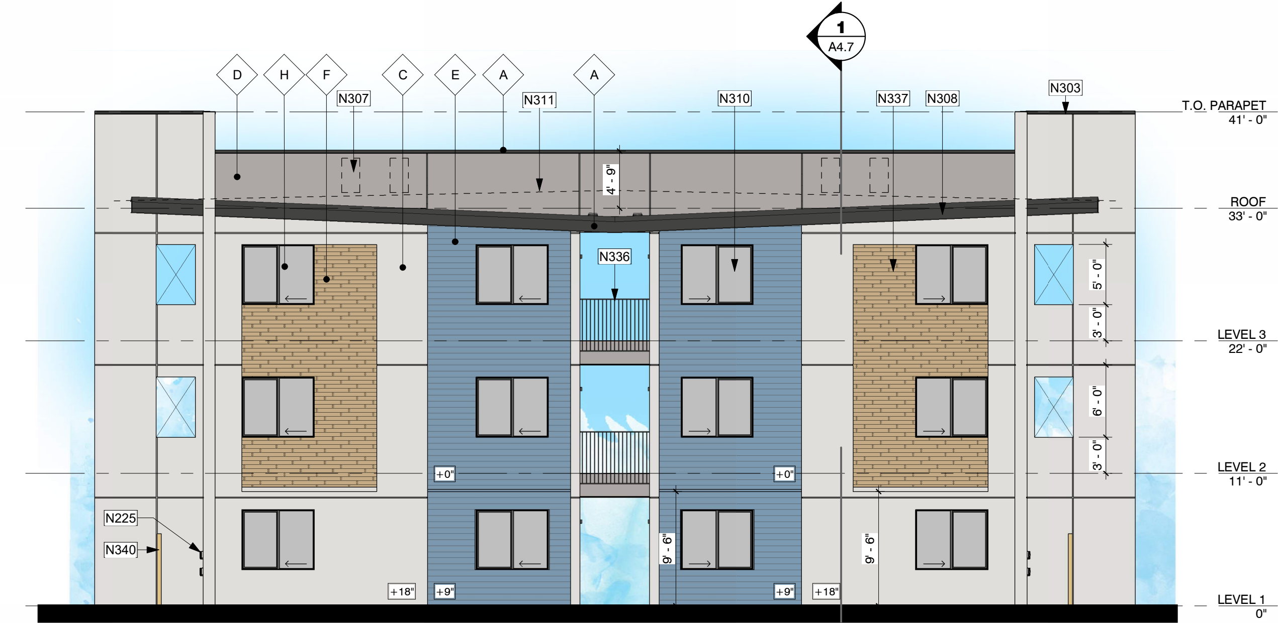
4 Building Type 3 - Elevation 4 1/8" = 1'-0"
