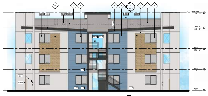
4 Building Type 2 - Elevation 4 1/8" = 1'-0"
