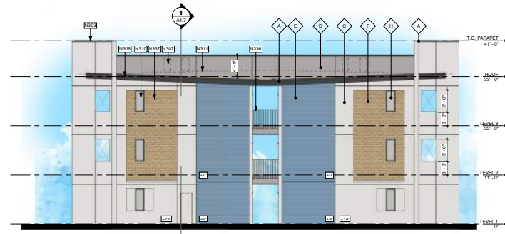
③ Building Type 3 - Elevation 3 1/8" = 1'-0"
